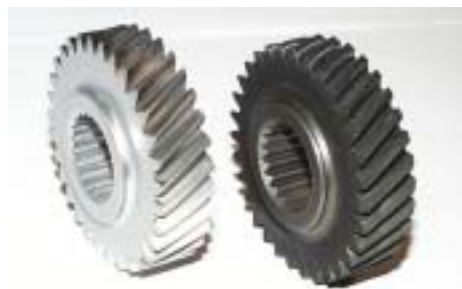
PM gear (left) and conventional helical gear (right) with inner spline used as a fixed gear in a standard gear box.
