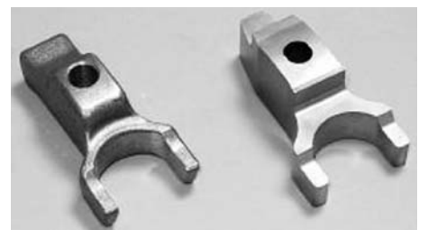
Injector yoke made by forging (left) and PM (right)
