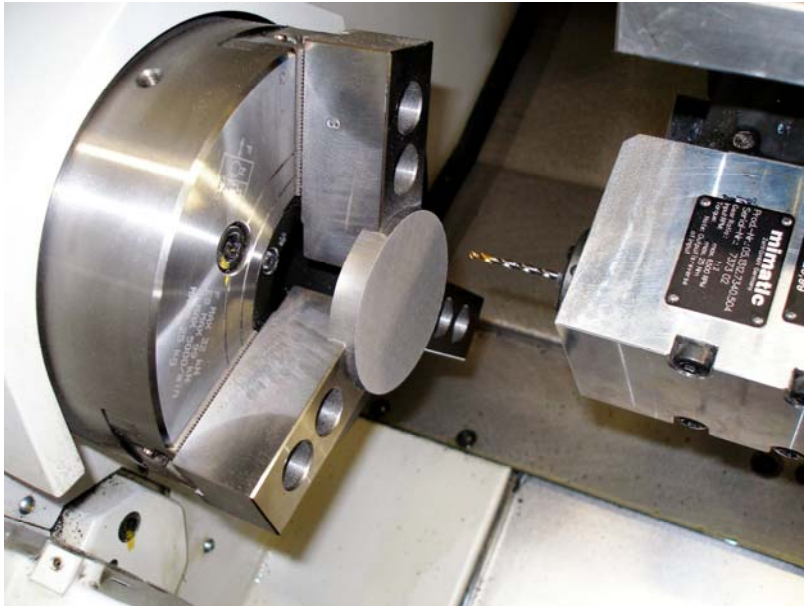
Fig. 2: Drilling operation in Mazak with Ø80 x 12 mm PM specimens
