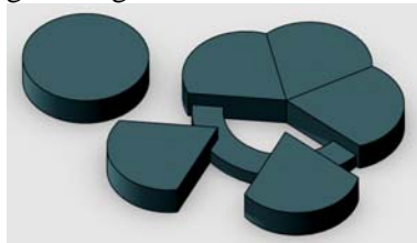
Figure 18: Larger structures made by machining and gluing segments together.
