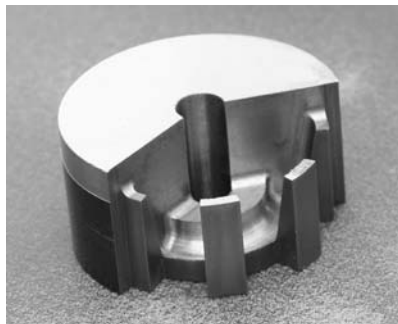
Figure 18: Claw pole structure being machined from Somaloy prototyping material.
