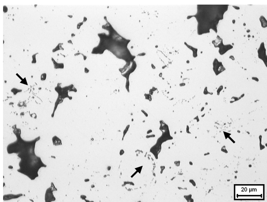
Trial 2: Sintering at 1120°C for 30 min.
