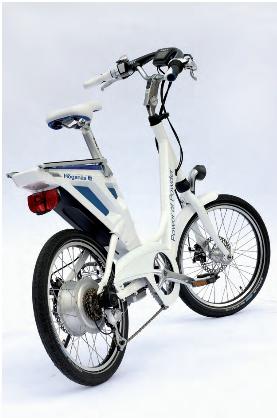
Höganäs PoP-bike with the Modulated Pole Machine mounted in the rear wheel
