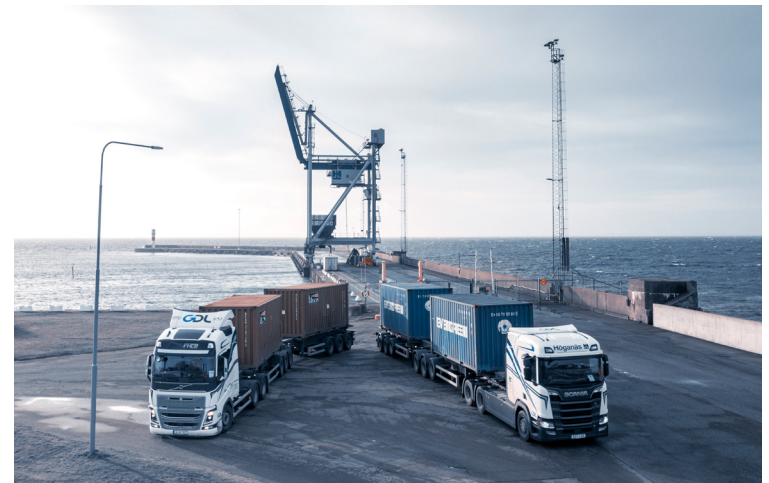
High-capacity vehicles may weigh a total of 74 tonnes instead of the normal 64 tonnes. For Höganäs, this means that we can drive with a double chassis and load two containers instead of one.
