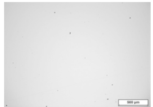
Non etched, as printed microstructure
