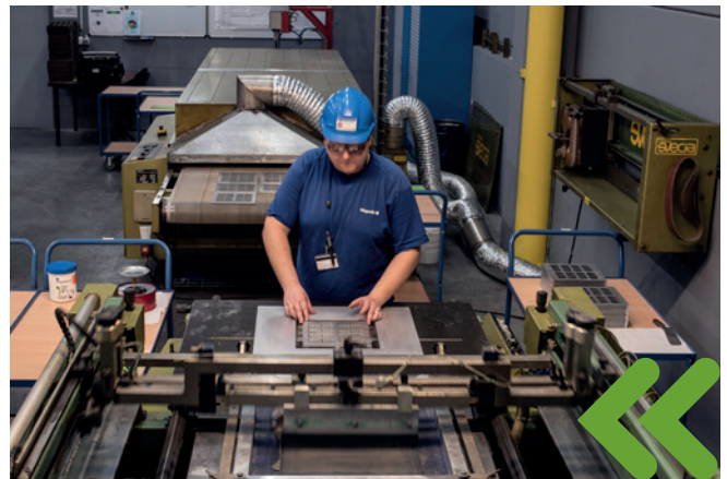
Höganäs screen printing process in Ath, Belgium.
