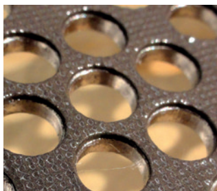
EGR hole-plate printed with Höganäs BrazeLet® Ni613P-9012 Nickel paste.
