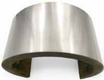
Shining surface without corrosion after 5000 hours salt spray test.
