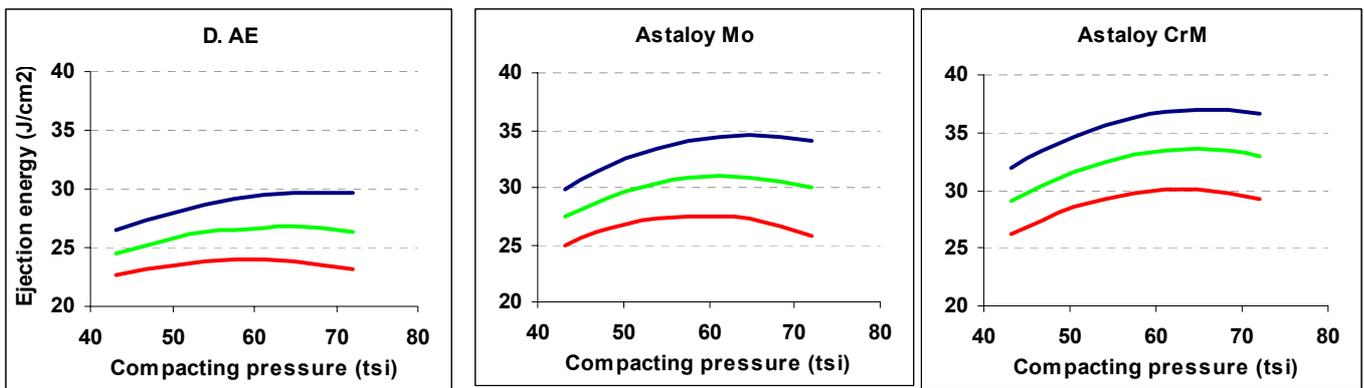
Figure 4: Ejection energies achieved using a die temperature of 60°C(140°F) and 0.30 – 0.60% Kenolube
