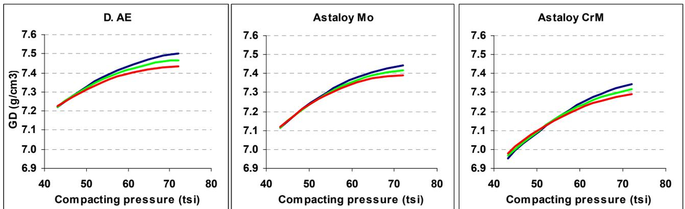
Figure 3: Green densities achievable using a die temperature of 60°C (140°F) and 0.30 – 0.60% Kenolube
