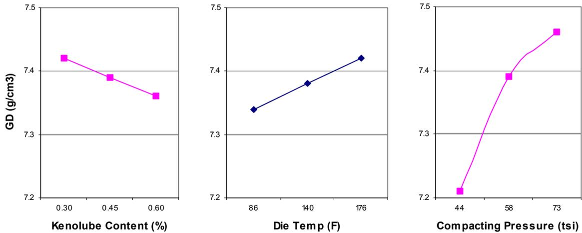
Figure 1: Effect of lubricant content, die temperature, and compacting pressure on the green density of D.AE + 0.3%C
