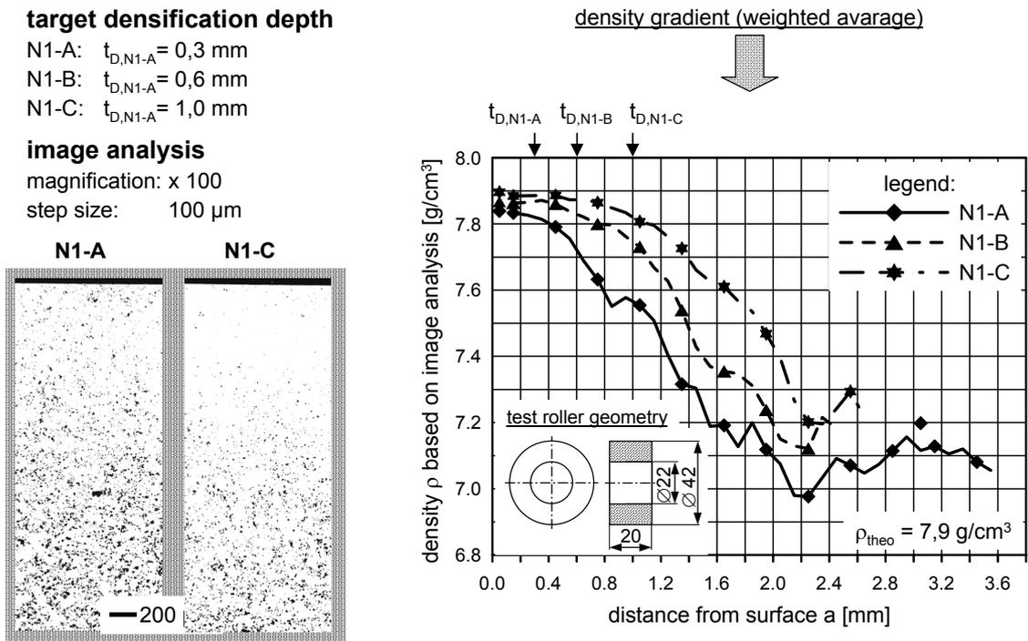
Figure 2. Density gradient measured by image analysis of variants N1-A,B,C
