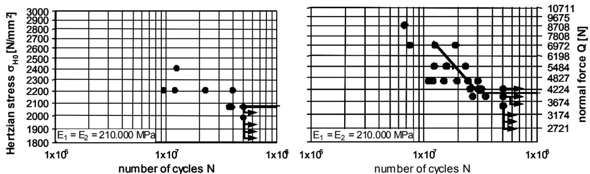
Figure 4. S/N diagrams of the reference material, 16MnCr5 (left) and the N3 material (right).
