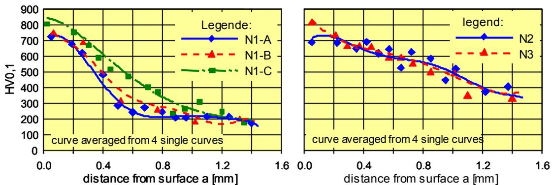
Figure 3. Micro hardness profiles of the tested materials.
