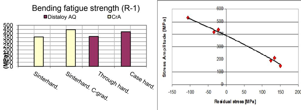
Figure 4, Residual stresses effect on fatigue properties
