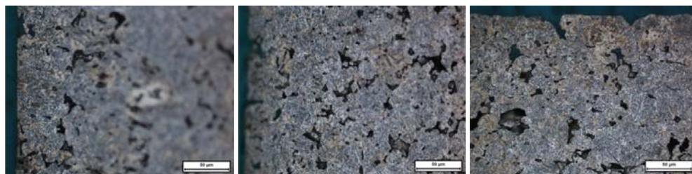
Figure 2. Surface carburization at different CO content
