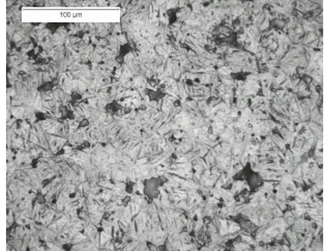
**Figure 5.** Microstructure of material B-2 (Astaloy CrM + 0.45% graphite, high temperature sintering and rapid cooling). Etched with Nital/Pical.
