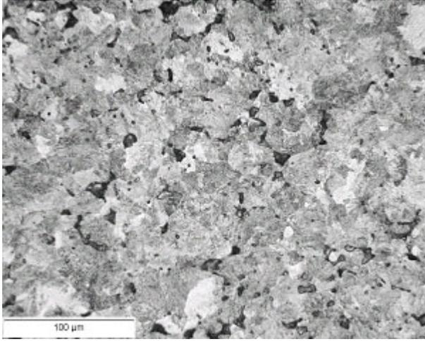
**Figure 4.** Microstructure of material A-1 (Astaloy CrL + 0.8% graphite, conventional sintering). Etched with Nital/Pical.
