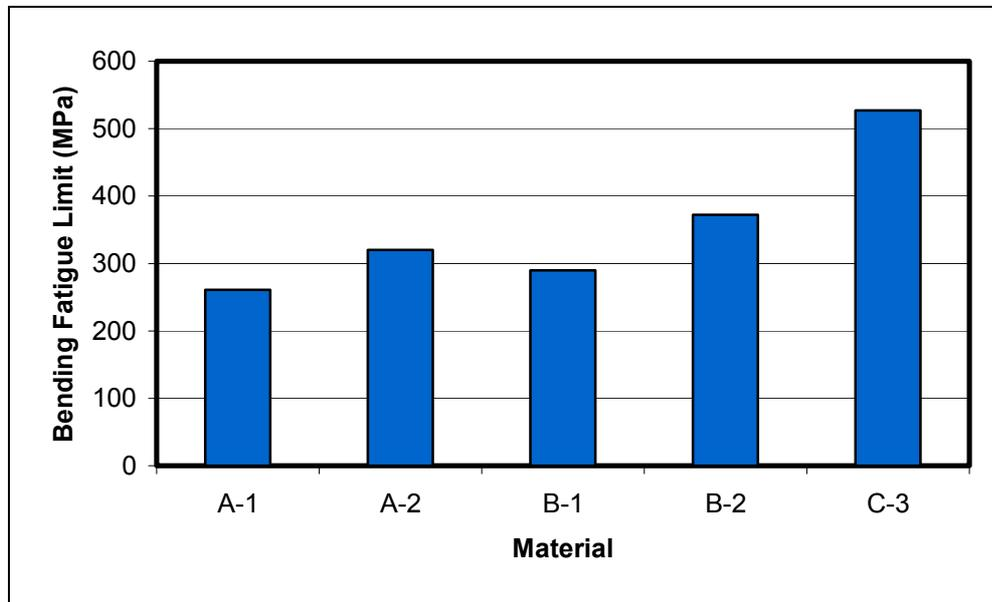
**Figure 1.** Plane bending fatigue limits of Cr-alloyed PM steels after different process routes.
