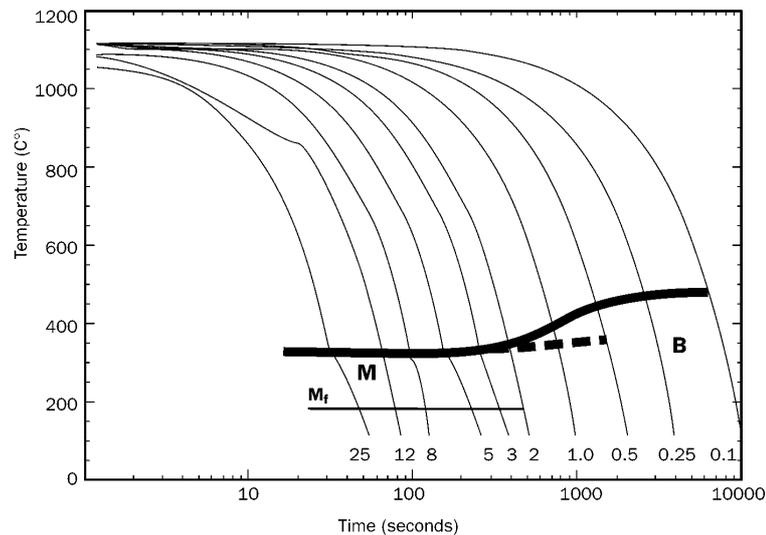
**Figure 6.** CCT diagram for Astaloy CrM + 0.4% C (B = Bainite, M = Martensite).
