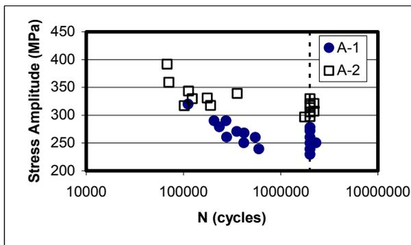
**Figure 2.** S-N diagram for materials A-1 & A-2 at fully reversed loading in plane bending.
