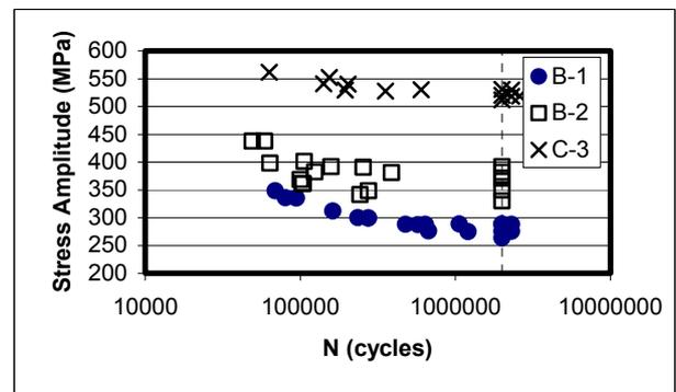
**Figure 3.** S-N diagram for materials B-1, B-2 & C-3 at fully reversed loading in plane bending.
