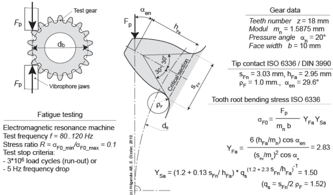
**Figure 1.** Tooth Root Bending Fatigue Schematic
