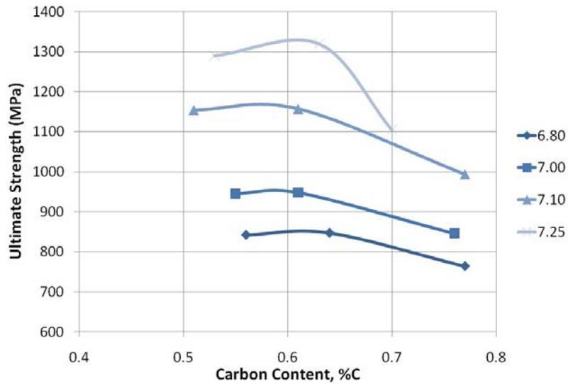
**Figure 4.** Tensile strength of D.A.Q as heat treated
