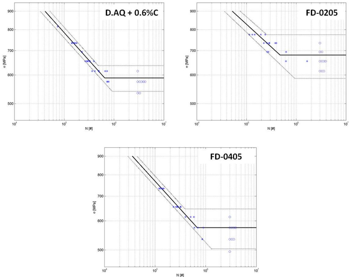
**Figure 8.** Gear Tooth Bending Fatigue SN Curves for Tested Material Systems
