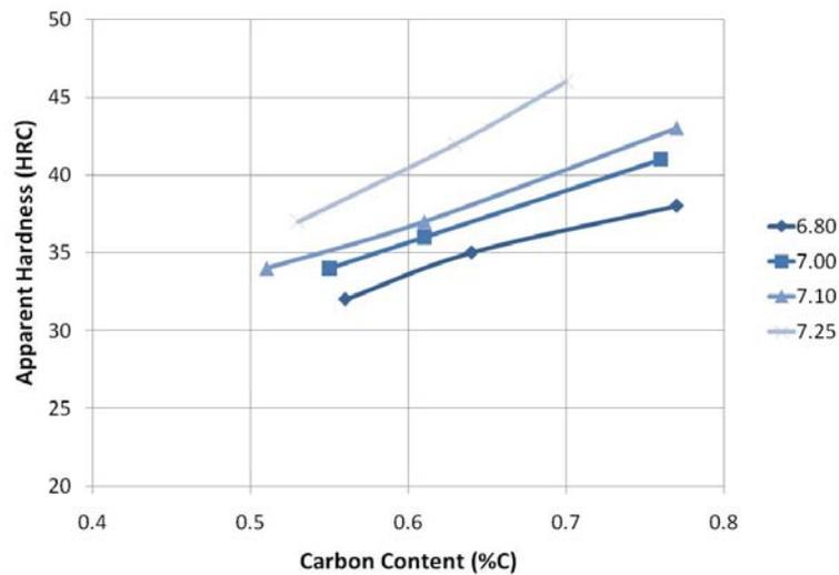
**Figure 3.** Apparent Hardness of D.AQ as heat treated
