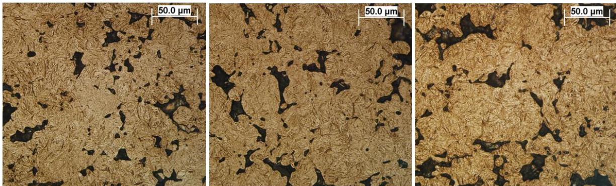
**Figure 2.** Microstructure Photographs (Left to Right: Mix 1, 2, & 3)
