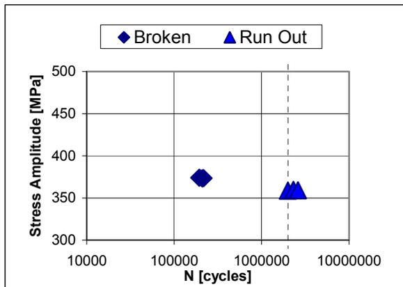
Fig. 2. Bending fatigue strength of vacuum carburized material A sintered at 1120°C (2050°F) (2350°F)
