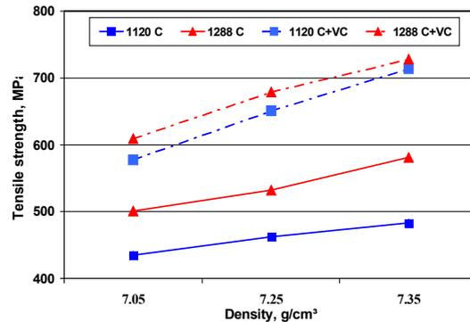
Figure 1. Tensile strength of material A after sintering and vacuum carburizing
