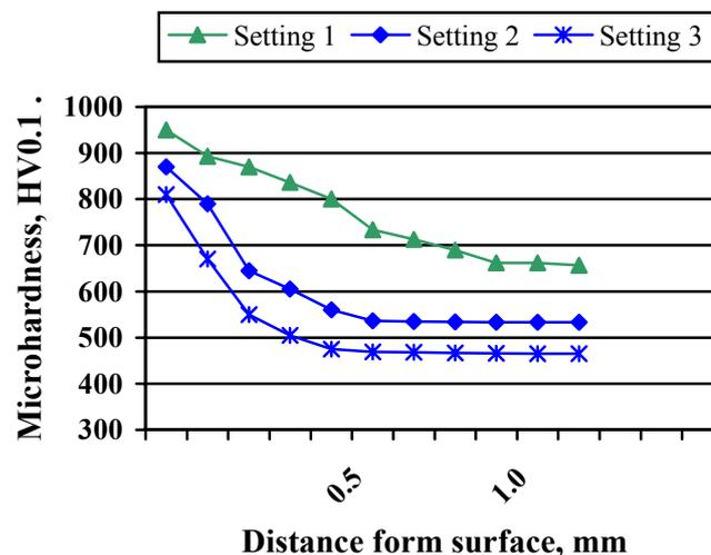
Figure 2. Micro hardness profiles obtained after vacuum carburization of material A with different parameters (density 7.25 g/cm<sup>3</sup>).
