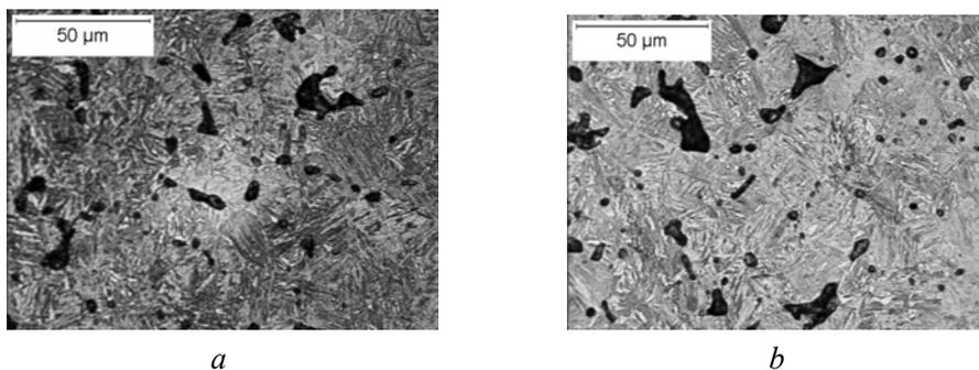
Figure 11. Material B, high-temperature sintered and vacuum carburized: *a* – surface; *b* – center.
