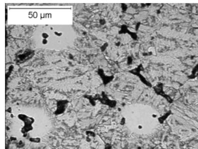
Fig. 9. Material B sintered at  $1288^\circ\text{C}$  ( $2350^\circ\text{F}$ ).
