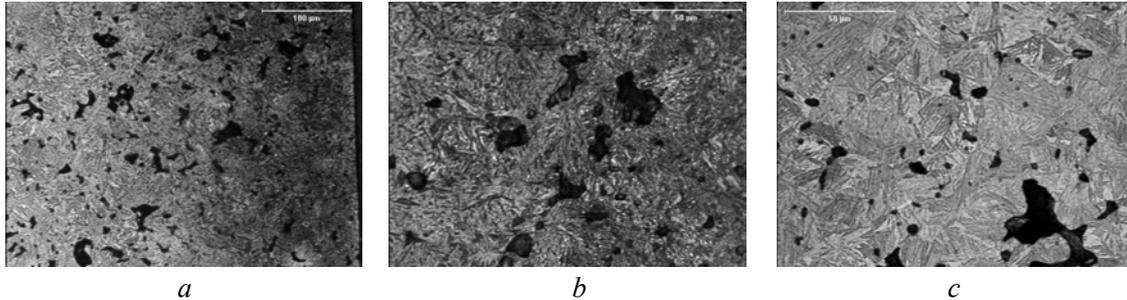
Figure 10. Material A, high-temperature sintered and vacuum carburized: *a* and *b* – surface, *c* – center.
