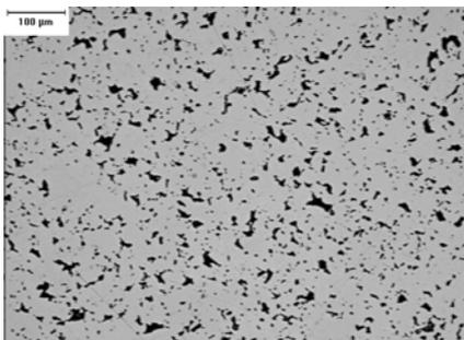
Fig. 4. Microstructure of material A sintered at 1120°C (2050°F).
