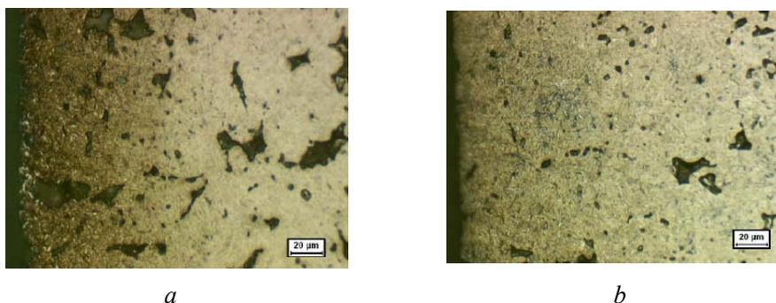
Figure 12. Material A sintered at  $1120^\circ\text{C}$  ( $2050^\circ\text{F}$ ) and vacuum carburized: *a* – oil quenched, *b* – gas quenched.
