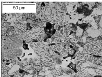
Fig. 8. Material B sintered at  $1120^\circ\text{C}$  ( $2050^\circ\text{F}$ ).
