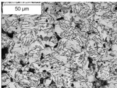
Fig. 6. Material A sintered at  $1120^\circ\text{C}$  ( $2050^\circ\text{F}$ ).
