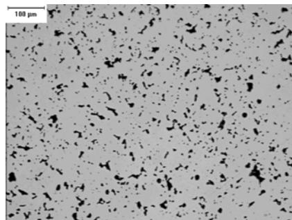
Fig. 5. Microstructure of material A sintered at 1288°C (2350°F).
