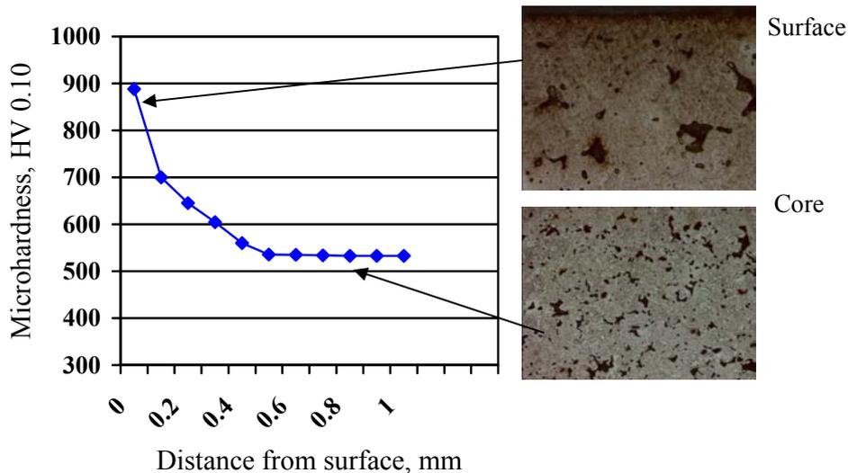
Fig. 15. Micro hardness and microstructure of vacuum carburized spur gear.
