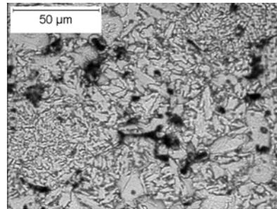
Fig. 7. Material A sintered at  $1288^\circ\text{C}$  ( $2350^\circ\text{F}$ ).
