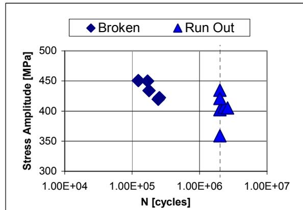
Fig. 3. Bending fatigue strength of vacuum carburized material A sintered at 1288°C
