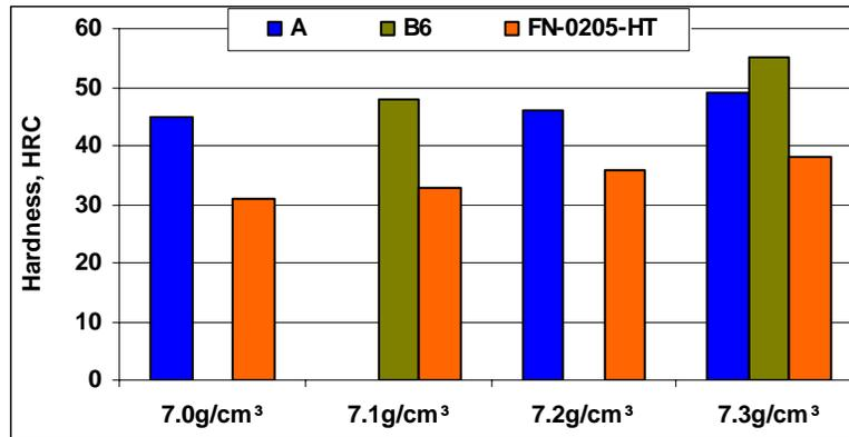
Figure 4. Hardness of Astaloy CMN in the heat treated condition compared to FN-0205-HT.
