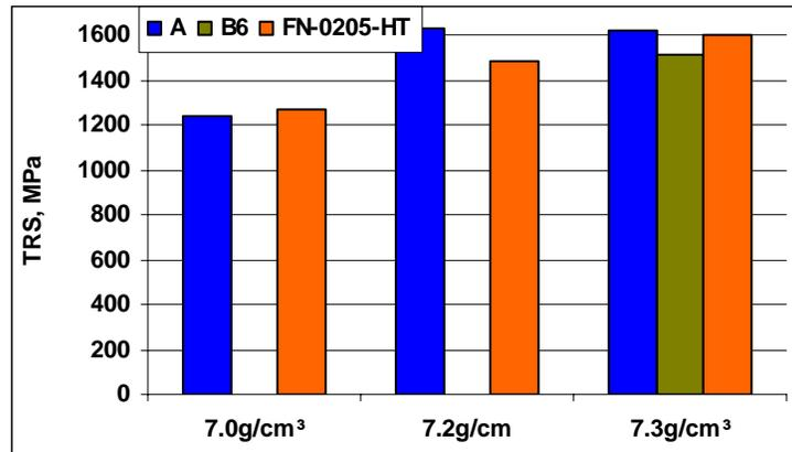
Figure 8. TRS at different densities compared to FN-0205-HT.
