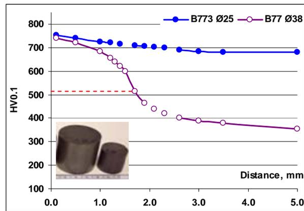
Figure 7. microindentation hardness of material B7 after through.
