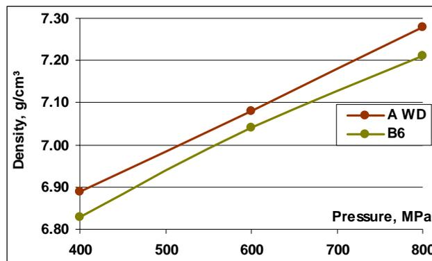
Figure 2. Compressibility curves of Astaloy CMN: AWD– heated die, B6 – RT compaction;
