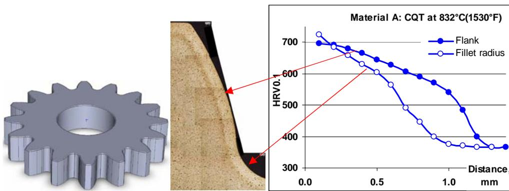
Figure 14. Microindentation hardness of case carburized spur gear.
