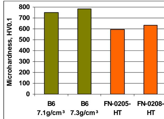
Figure 6. Microindentation hardness of material B.
