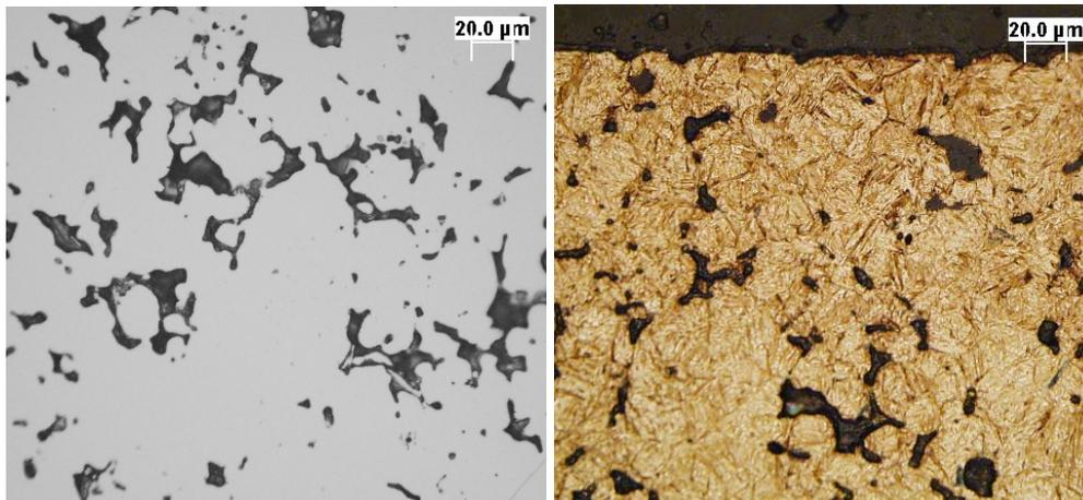
Figure 12. Typical unetched and etched microstructures of materials A (surface) and B.
