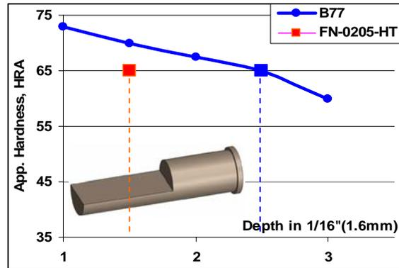
Figure 11. Jominy hardenability tests compared to FN-0205-HT.
