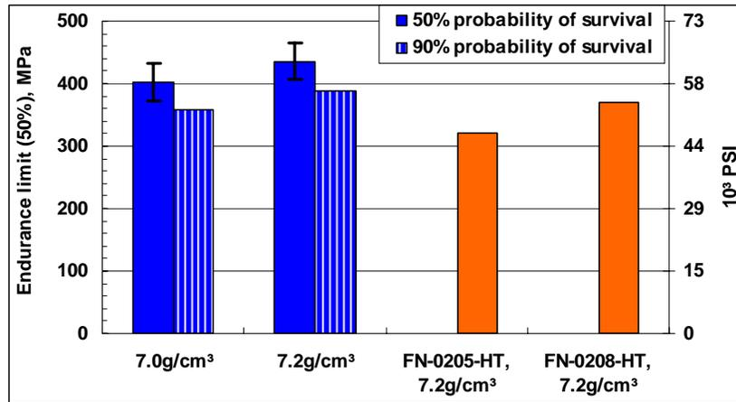
Figure 10. Fatigue limit of the case carburized material A at 50 and 90% probability of survival.
