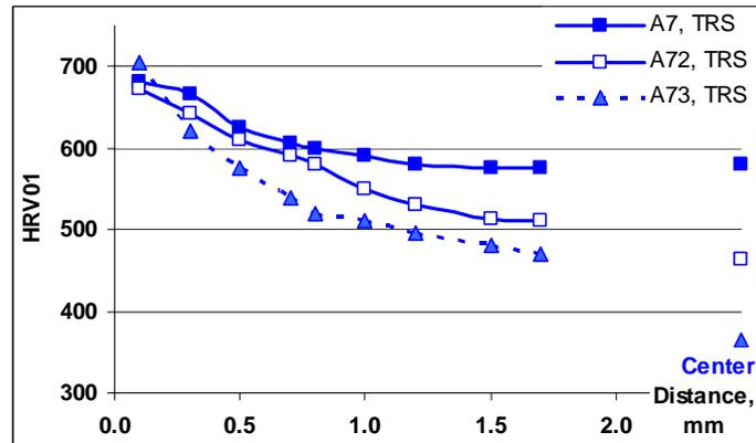
Figure 5. Microindentation hardness (100g load) of carburized material A.
