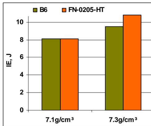
Figure 9. Impact Energy of material B6 compared to FN-0205-HT.
