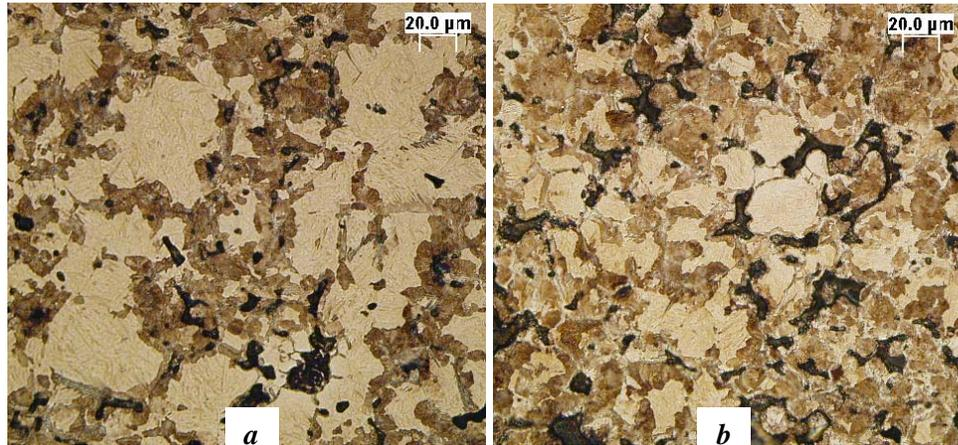
Figure 13. Material B7 microstructures in center areas: *a* – cylinder Ø25mm; *b* – Ø38mm.
