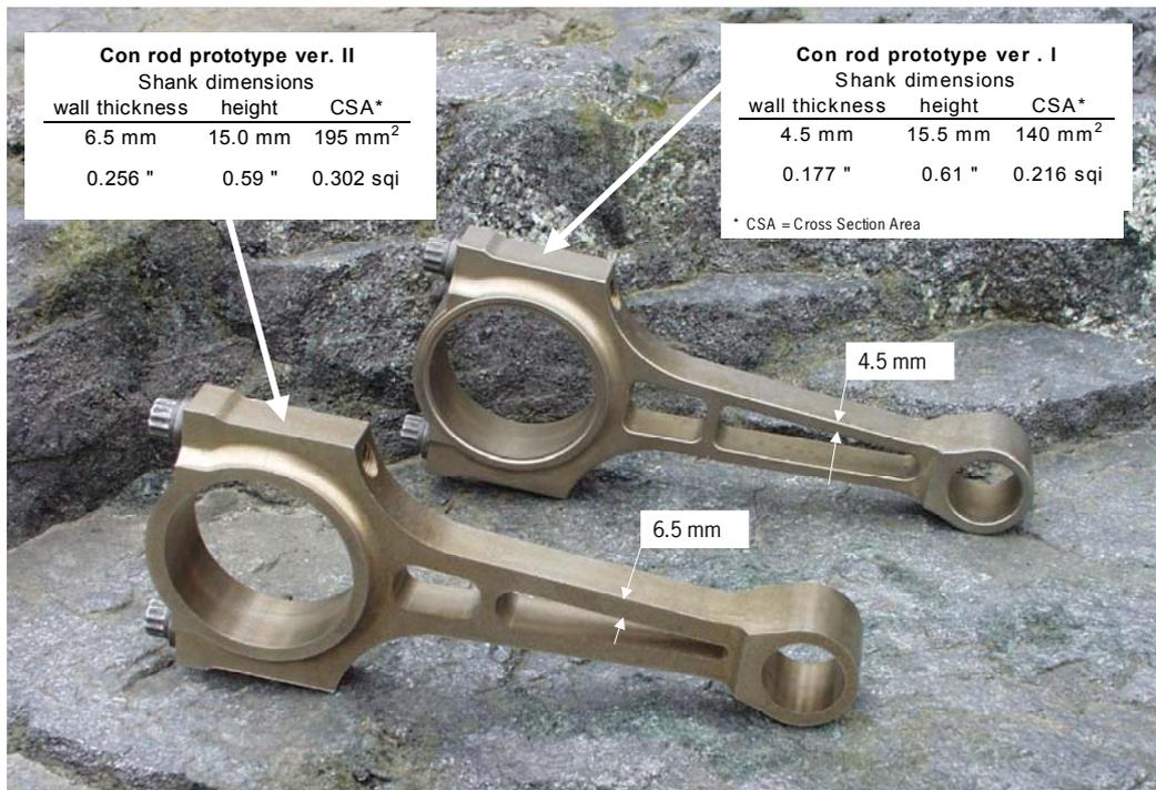
**Figure 8.** Re-design of Warm Compacted prototype connecting rod
