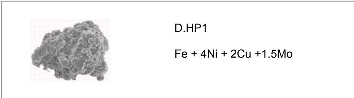
**Figure 4.** Diffusion alloyed powder type D.HP1
