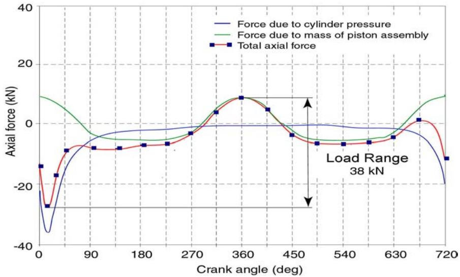
**Figure 2.** Connecting rod forces at engine peak power
