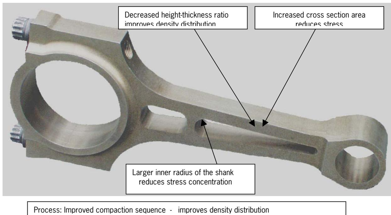
**Figure 7.** Design- and process improvements of prototype con rod –II
