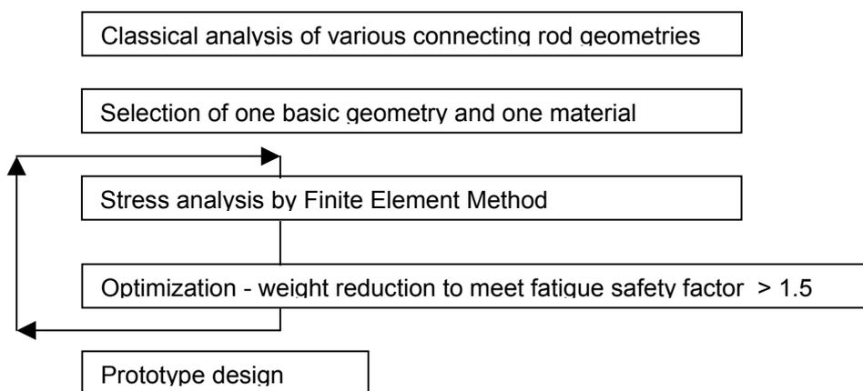
**Figure 6.** Design route for prototype connecting rod (first version)
