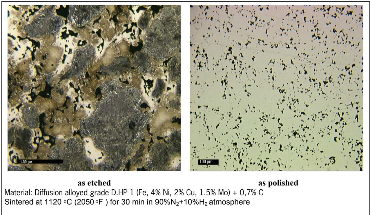
**Figure 5.** Metallographic structure of Warm Compacted and sintered connecting rod material
