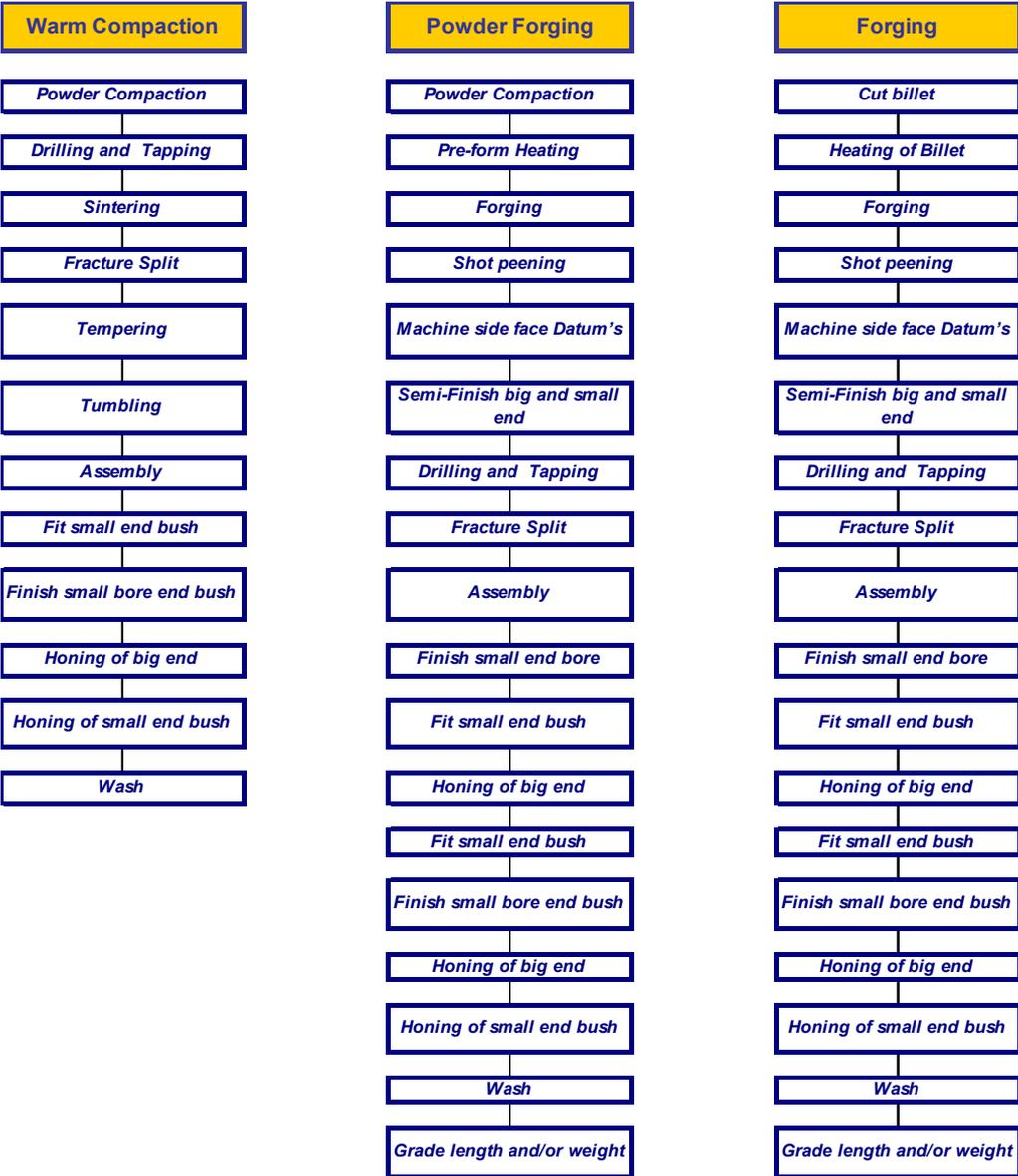
Figure 3. Processing route for connecting rods
