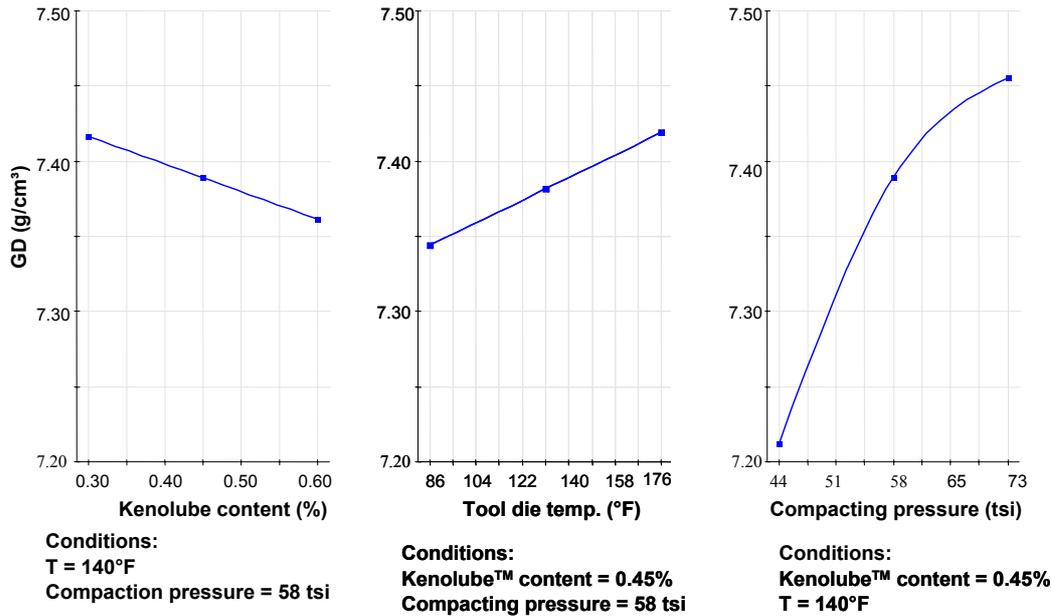
Figure 3. Influence of lubricant amount, die temperature and compaction pressure on the green density for D.AB + 0.3% combined carbon content.
