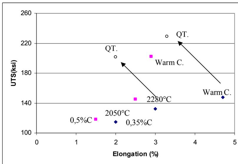
Figure 5. Effect of sintering temperature, increased density and quenched and tempered on Astaloy CrM.
