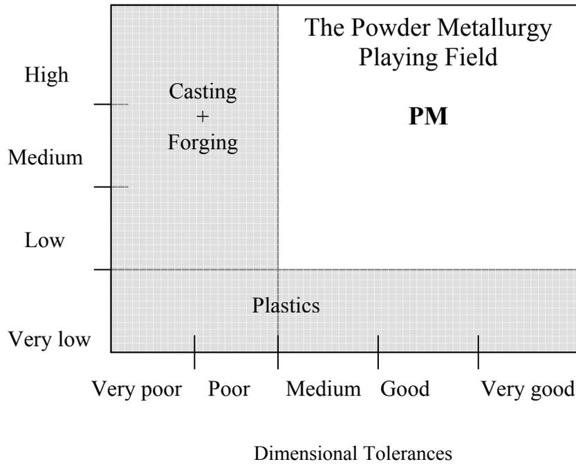
Figure 1. Definition of “Powder Metallurgy Playing Field” related to mechanical strength and dimensional tolerances
