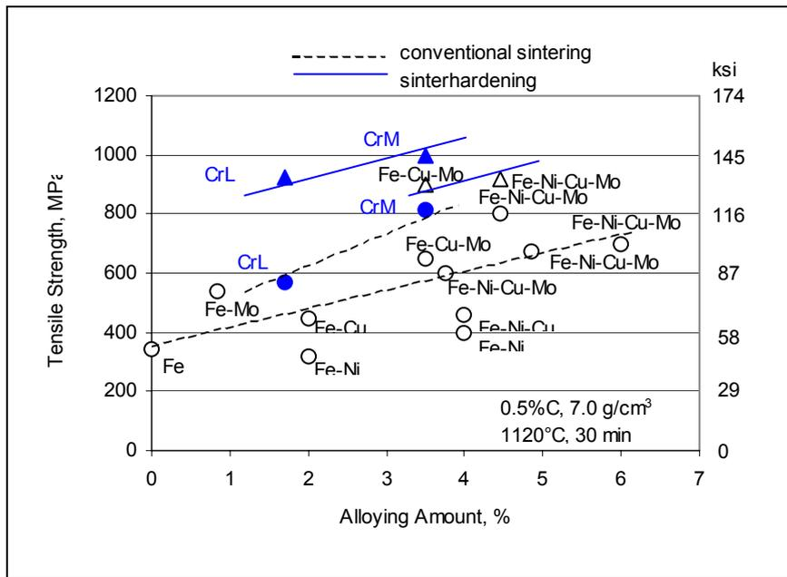
Figure 6. Comparison tensile strength and alloying amount.
