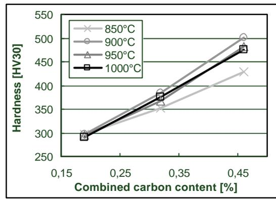
**Fig.2b:** cold compacted, sintered at 1250°C
