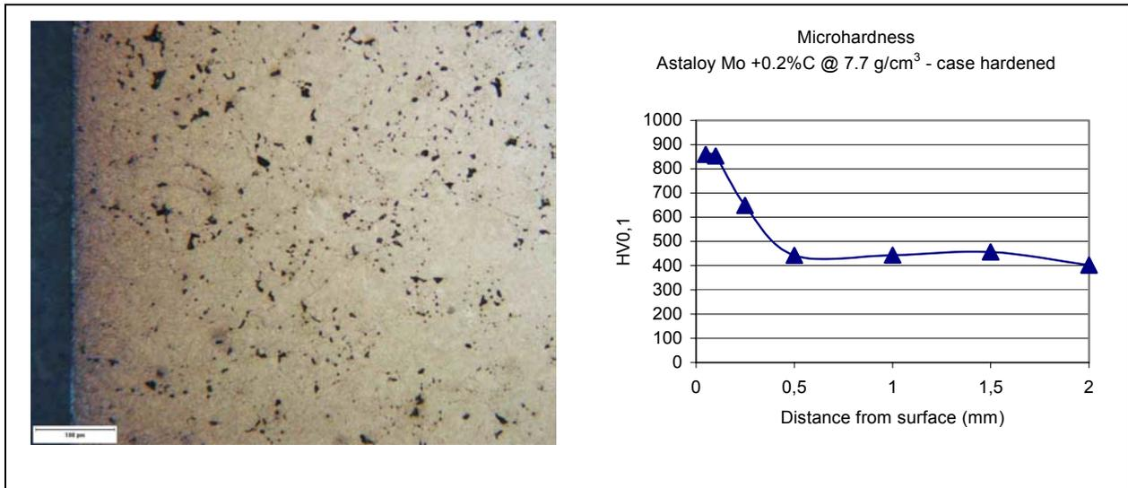
Figure 10. Micrograph and hardness profile for case-hardened test bar. Astaloy Mo+0.2%C @ 7.7g/cm<sup>3</sup>
