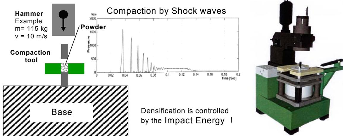
Figure 4. Basic mechanism of HVC and Hydropulsor HYP35-4 impact machine (4 kJ maximum compaction energy; 2 950 ft lb) with automatic tool adapter
