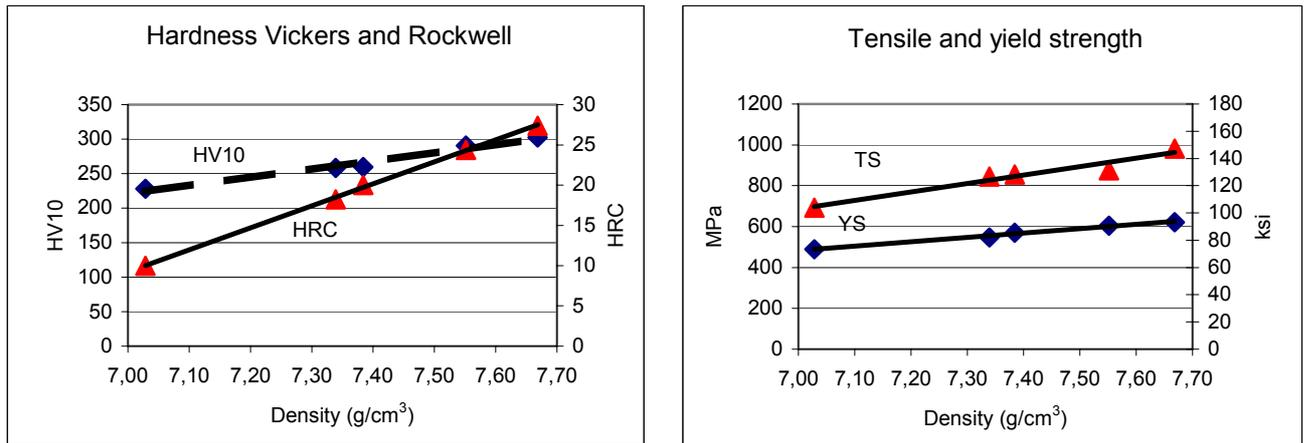
Figure 7. Mechanical properties of AstaloyMo +2%Ni +0.6%C sintered at 1120°C (2050°F) in 90%N<sub>2</sub>/10%H<sub>2</sub>
