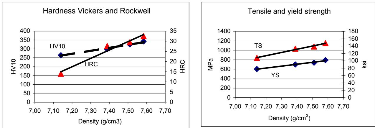
Figure 9. Mechanical properties of Astaloy CrM + 0.4%C sintered at 1120°C (2050°F) in 90%N<sub>2</sub>/10%H<sub>2</sub>
