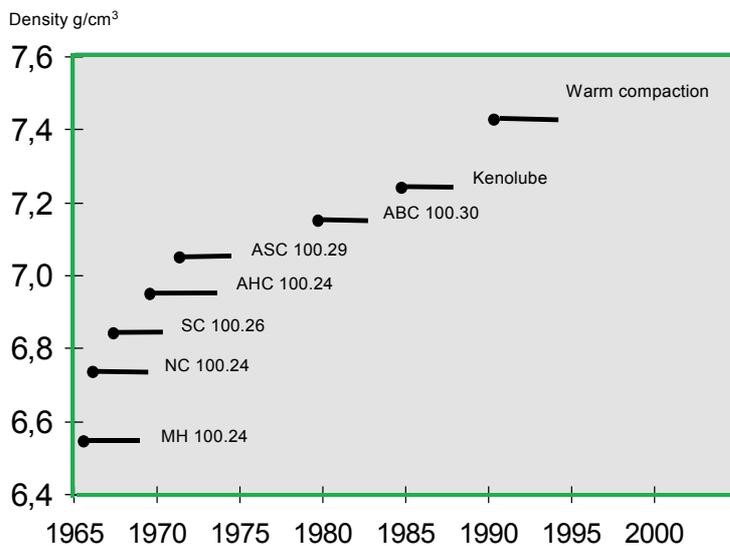
Figure 2. 30 years of density improvements in powder metallurgy
