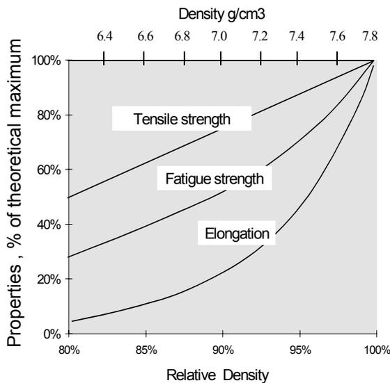
Figure 1. Principal materials properties relation to density for sintered ferrous steel
