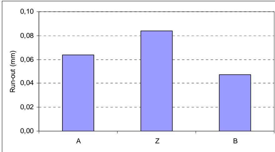
Figure 13: Average run-out of the sintered parts
