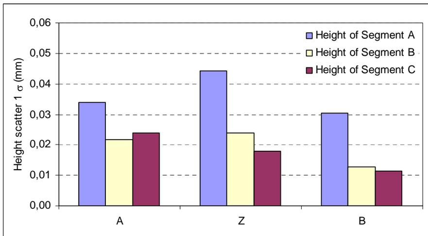
Figure 12: Total scatter in height of the sintered parts
