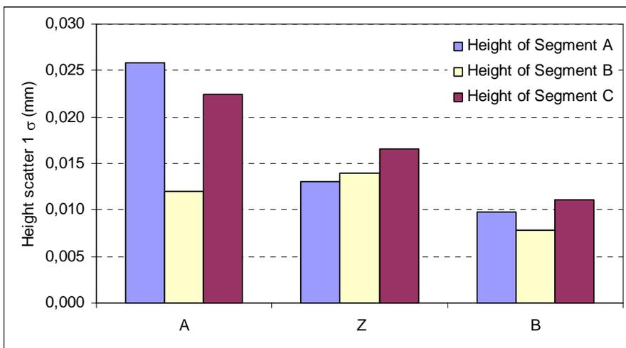
Figure 10: Scatter in height of each segment of the sintered parts
