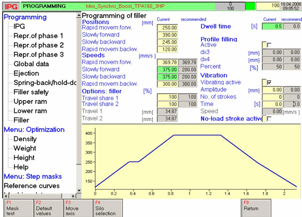
Figure 4: IPG® interface – six phase filler program
