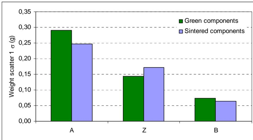
*Figure 8: Weight scatter of green and sintered parts*
