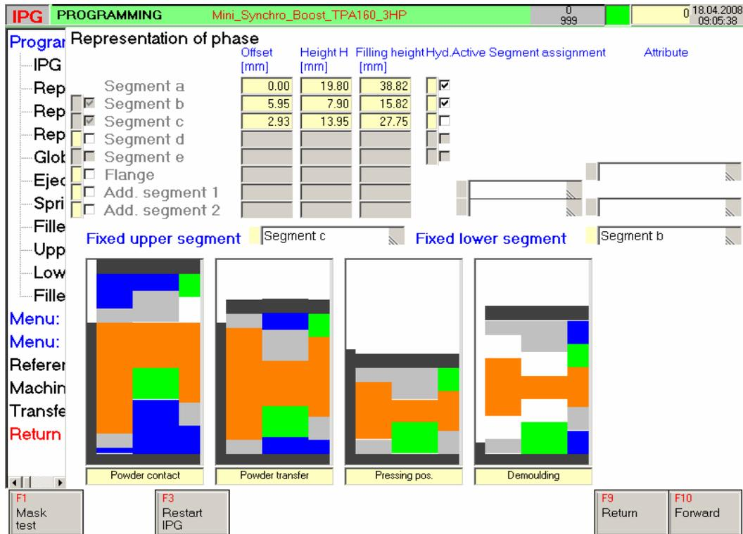
Figure 3: Press control software IPG® interface
