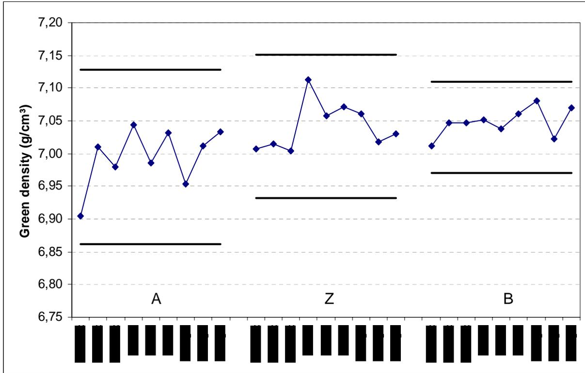
Figure 9: Green density of segments, measured values and  $\pm 3 \sigma$
