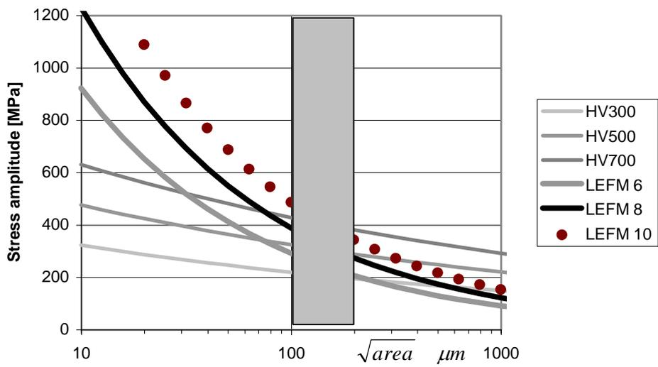
Fig. 3. Combined diagrams for the LEFM and the modified Murakami models valid for surface pores. The shadowed area show typical defect sizes found by fractography in PM steel at densities around  $7.3 \text{ g/cm}^3$ .
