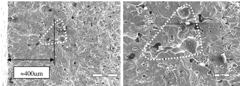
**Fig.1.** Crack initiation site in shot-peened AstaloyCrL subjected to axial fatigue. The dotted line outlines the convex envelope (marked with dotted line) of the projected initial defect. The defect area is approximately  $20.000 \mu\text{m}^2$ . The bars are  $200\mu\text{m}$  (left) and  $50\mu\text{m}$  (right) respectively.
