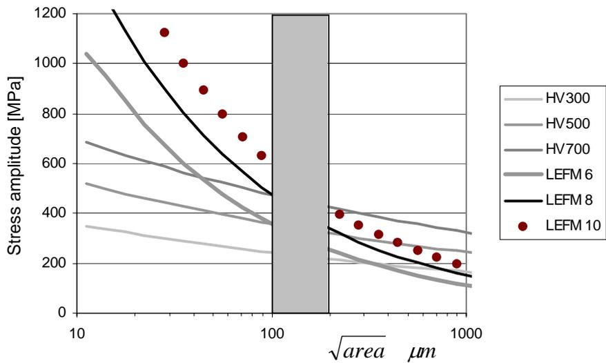
Fig. 2. Combined diagrams for the LEFM and the modified Murakami models valid for internal pores. The shadowed area show typical defect sizes found by fractography in PM steel at densities around  $7.3 \text{ g/cm}^3$ .
