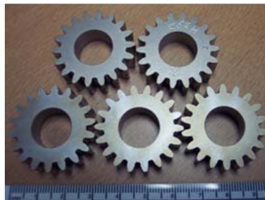
Figure 12. Spur gear used for case carburization study.
