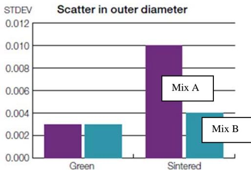
Fig. 4. Dimensional scatter of outer diameter of VVT stator after compaction and sintering for mix A and B.
