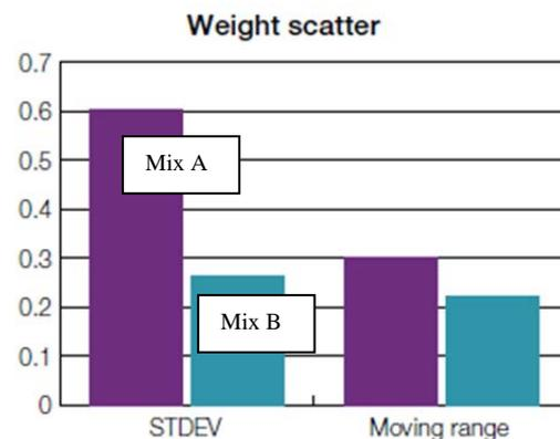
Fig. 3. Weight scatter of VVT stator obtained with Mix A and Mix B
