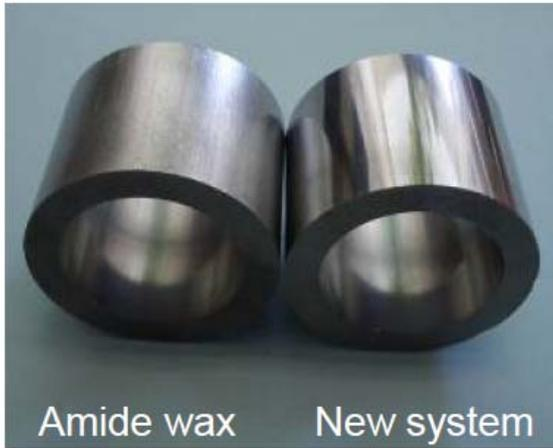
Figure 14. Components after compaction
