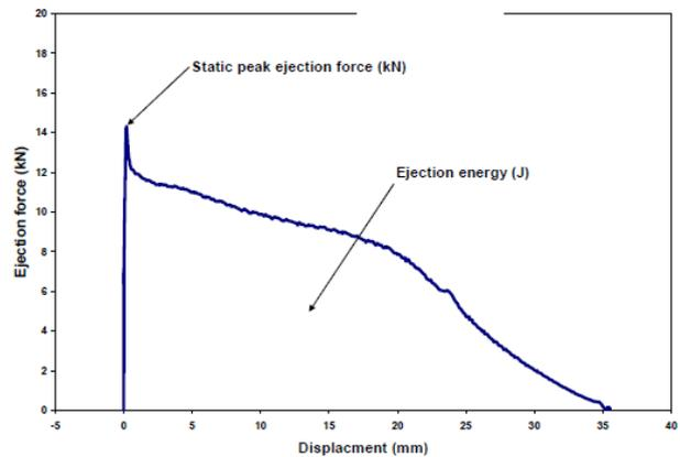
Figure 4 The force (kN) measured during the ejection of a component
