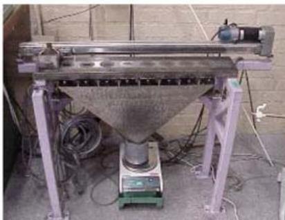
Figure 2. The die filling equipment
