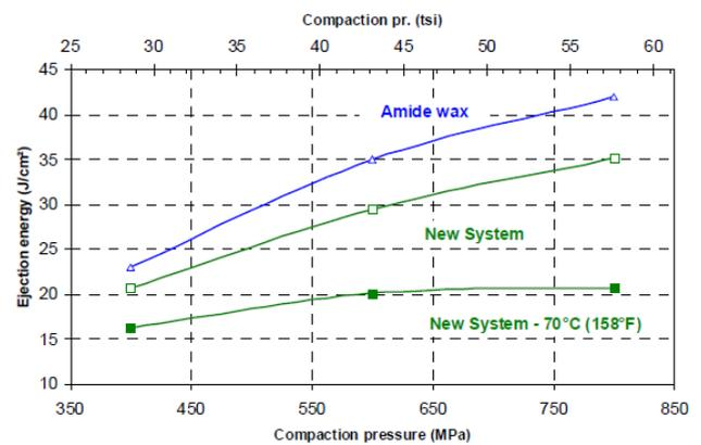
Figure 8. Ejection energy
