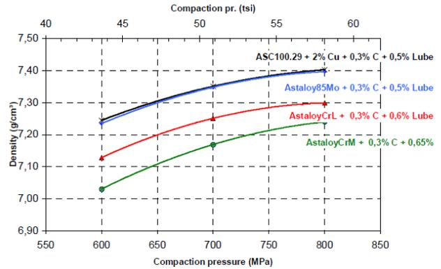
Figure 12. Densities with new system in combination with different iron powders.
