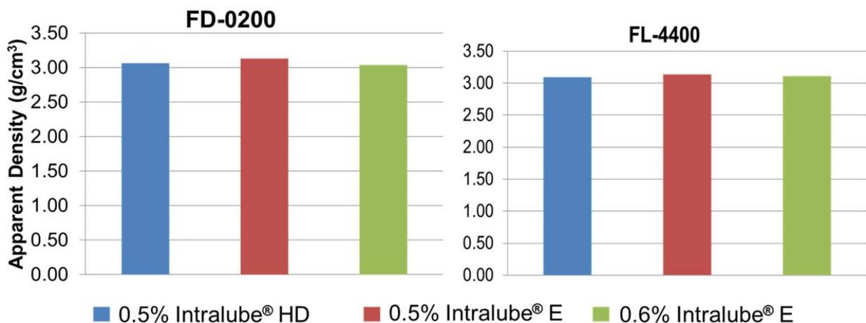
**Figure 5:** Apparent density of Intralube® HD mix verse Intralube® E mix
