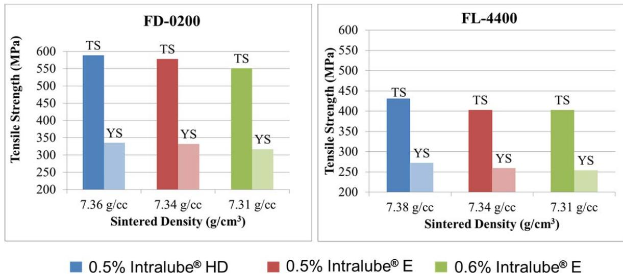
**Figure 9:** Tensile and yield strength properties of Intralube® E vs. Intralube® HD at 750Mpa
