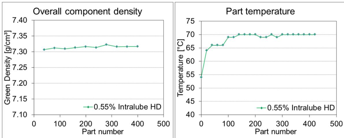
**Figure 17:** a.) Green density scatter of helical gears after ejection over 400 parts b.) Temperature scatter of helical gears after ejection over 400 parts
