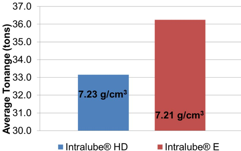
**Figure 13:** Average compaction tonnage at similar green densities
