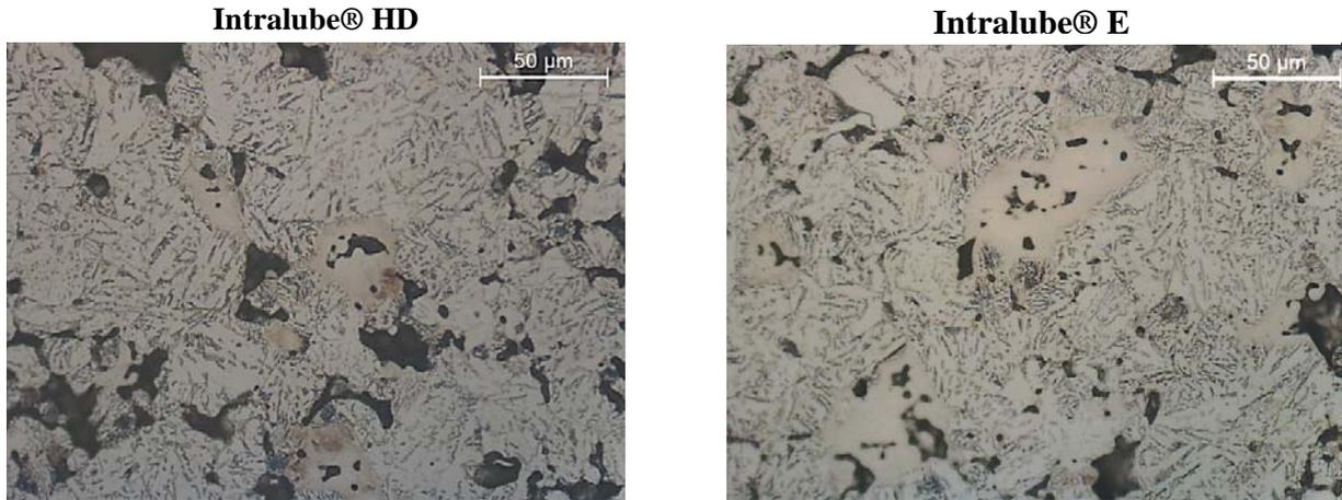
**Figure 14:** Microstructures of FLN-4205 shift weight components
