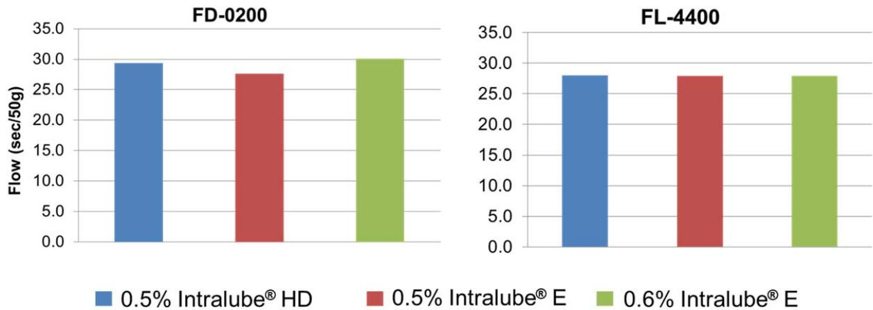
**Figure 6:** Flow of Intralube® HD mix versus Intralube® E mix
