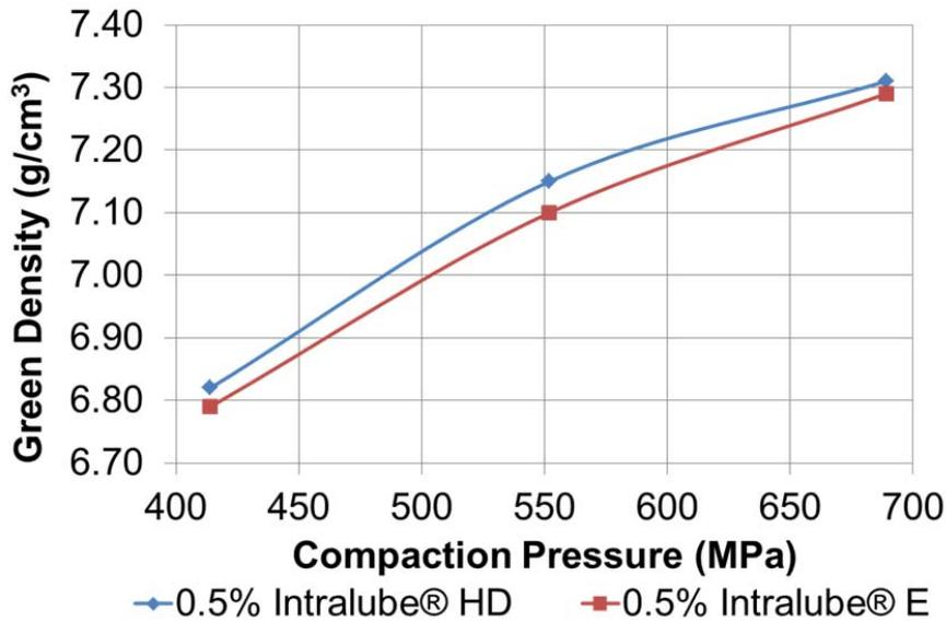
**Figure 12:** Compressibility Curve of FLN-4205 mixes with Intralube® HD and Intralube® E
