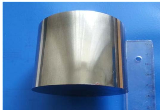
**Figure 11:** Compacted cylinder (64 mm diameter) of the mix D.AB + 0.5% Intralube® HD with a height of 50mm (part number 20).
