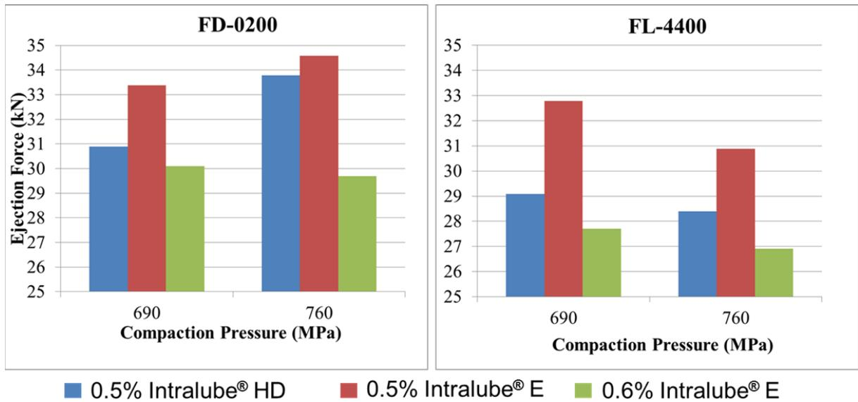
**Figure 8:** Ejection force properties of Intralube® E vs. Intralube® HD
