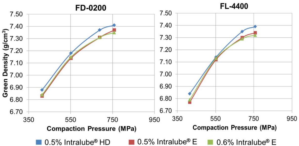
**Figure 7:** Compressibility curves of Intralube® E vs. Intralube® HD
