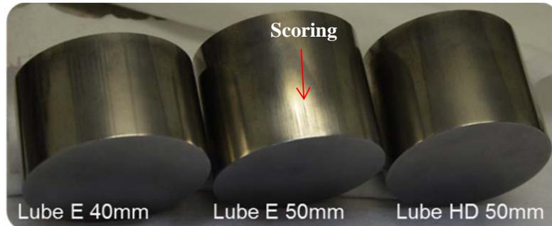
**Figure 10:** Maximum height test surface appearance of Intralube® E vs Intralube® HD
