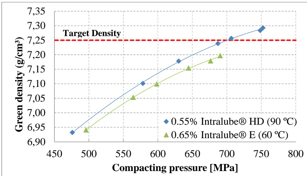
**Figure 15:** Helical gear compressibility curve
