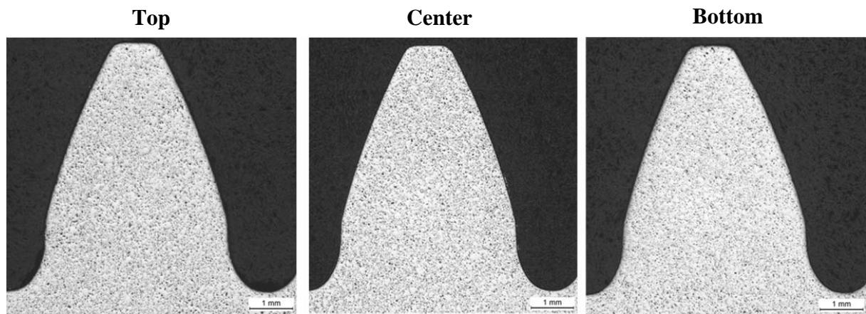
**Figure 18:** Horizontal cross section of helical gear tooth
