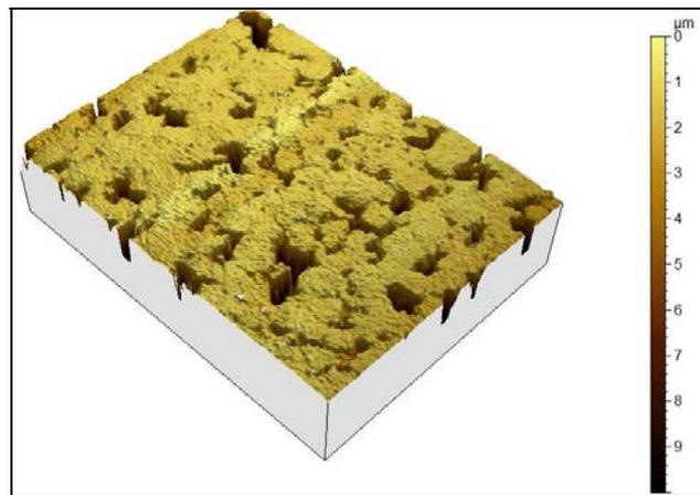
Figure 5. Sintered surface, press direction is parallel to the measured surface.
