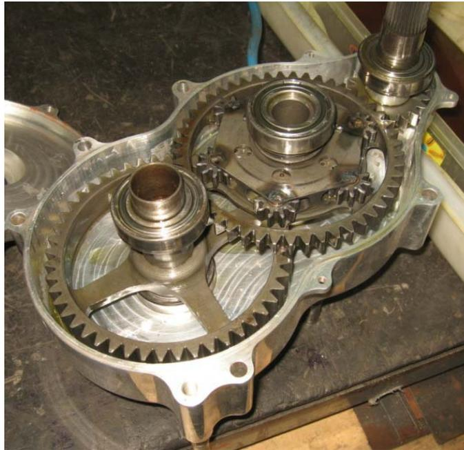
Figure 1. Redesigned HIP transmission made in sinter steel for a Baja vehicle
