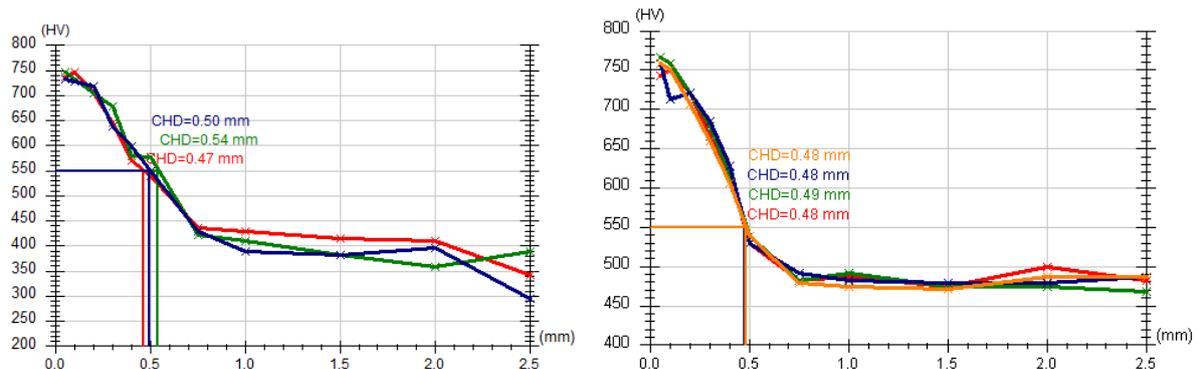
Figure 6. Left: Case profile for HIP FS bar
