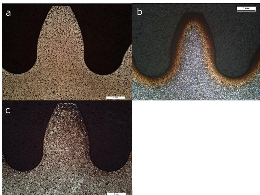
Figure 5. Microstructures, a. Astaloy Mo, b. Astaloy CrA and c. Distaloy AE.
