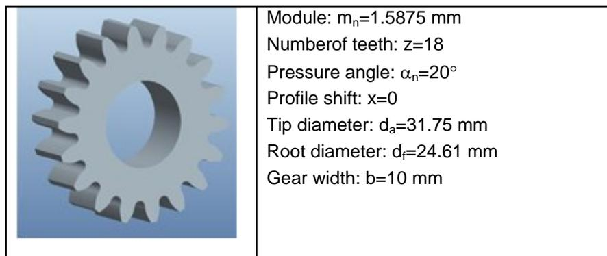
Figure 4. Gears used for the experiments.
