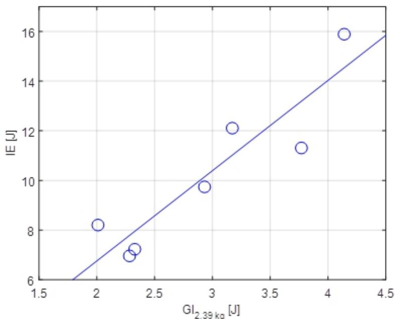
Figure 7. Comparison between gear impact energy and Charpy impact energy.
