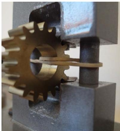
Figure 2. Sketch of gear specimen holder.
