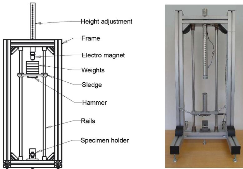
Figure 1. Sketch of the design of the test rig and photo of the actual implementation.
