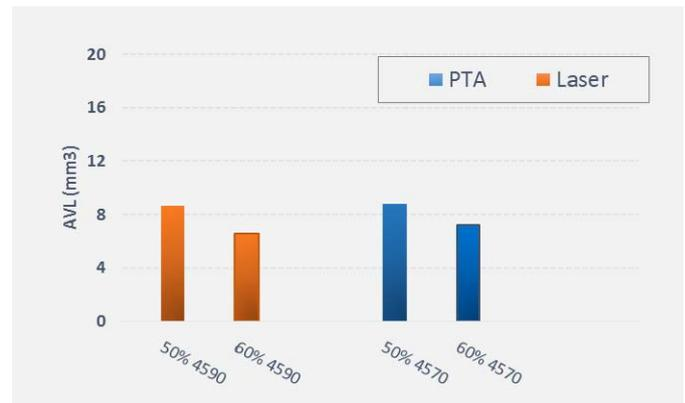
Figure 2. AVL ( $\text{mm}^3$ ) of laser cladded and PTA welded mixes based on 1559-40 with 50 respectively 60wt% tungsten carbides
