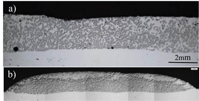
Figure 5. The micrographs show the distribution of the tungsten carbides in a) 1559-40+50wt% 4590, laser clad; b) 1559-40+50wt% 4570 welded as observed under a LOM.
