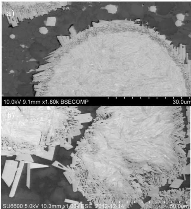
Figure 4. SEM-BSE photos showing different degree of dissolution of the tungsten carbides; a) 1559-40+50wt% 4590, laser clad; b) 1559-40+50wt% 4570, PTA welded
