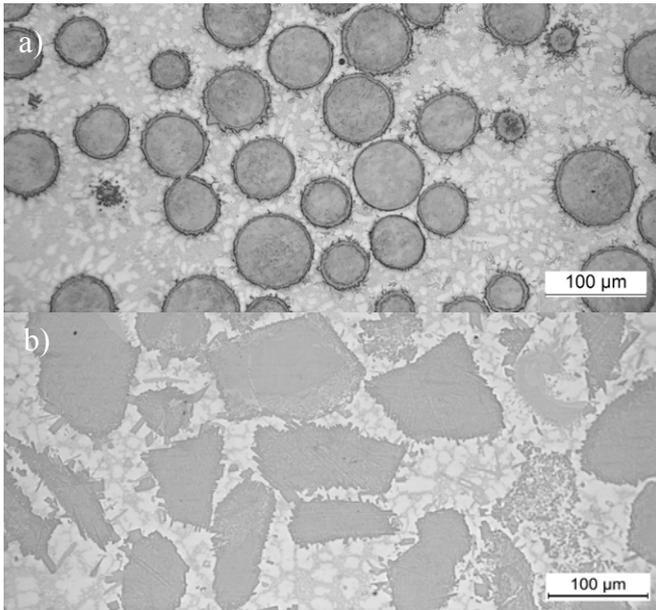
Figure 3. Microstructure of a) 1559-40+50wt% 4590, laser clad; b) 1559-40+50wt% 4570 welded as observed under a LOM.
