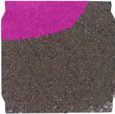
**Figure 3. Cross section of a test bar with the final fatigue crack marked.**
