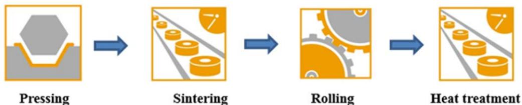
Figure 1. Production chain for a sintered and rolled component
