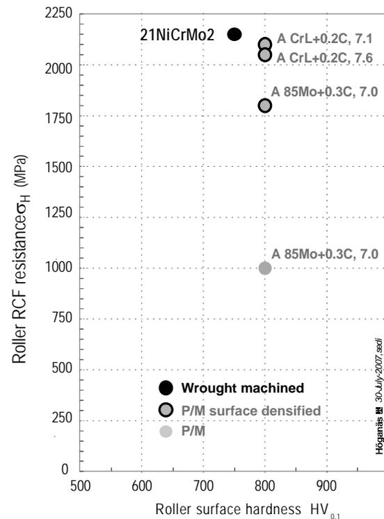
Figure 7. Roller RCF resistance (Hertzian stress).
