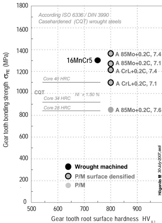
Figure 6. P/M gear tooth bending strength  $\sigma_{FE}$ .
