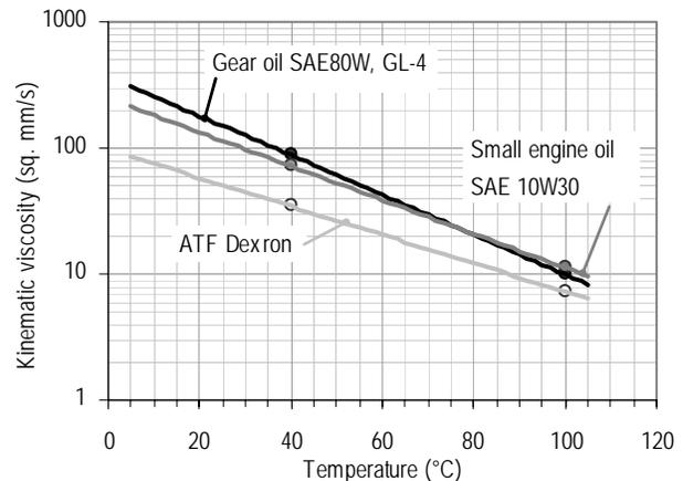
Figure 2. Viscosity vs. temperature for three typical oils in automotive applications.
