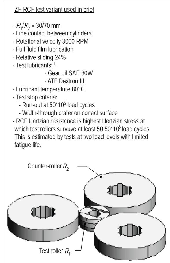
Figure 4. Illustration of the rollers' contact of the ZF-RCF test and some basic test data.
