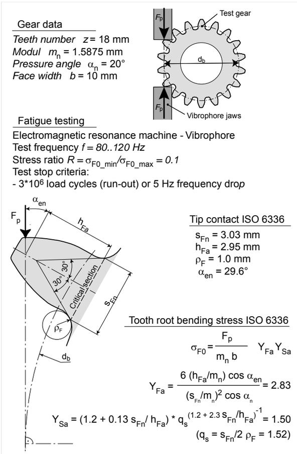
Figure 3. The prototype gear, basic facts about the gear tooth root bending testing and a brief schedule of gear bending stress calculations according to ISO 6336
