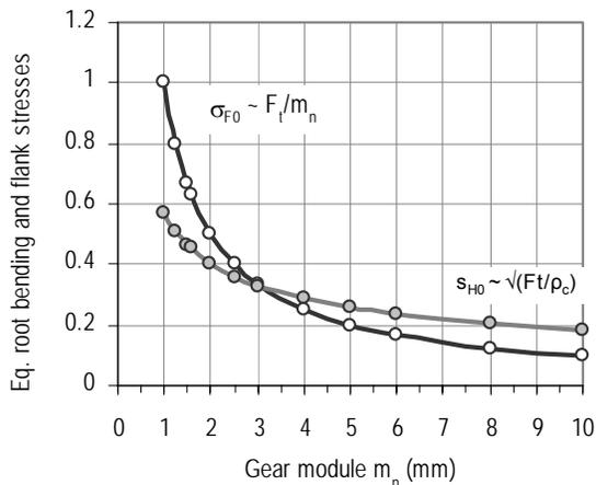
Figure 1. An approximation of equivalent gear tooth root bending and Hertzian flank stresses as a function of module.
