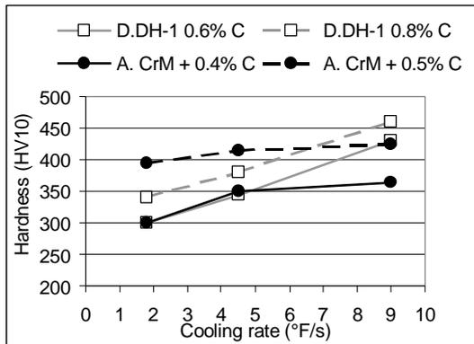
Figure 4, Hardness vs cooling rate
