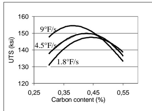
Figure 7. UTS vs cooling rate, Astaloy CrM
