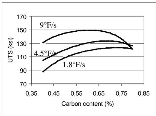
Figure 6. UTS vs cooling rate, D.DH-1
