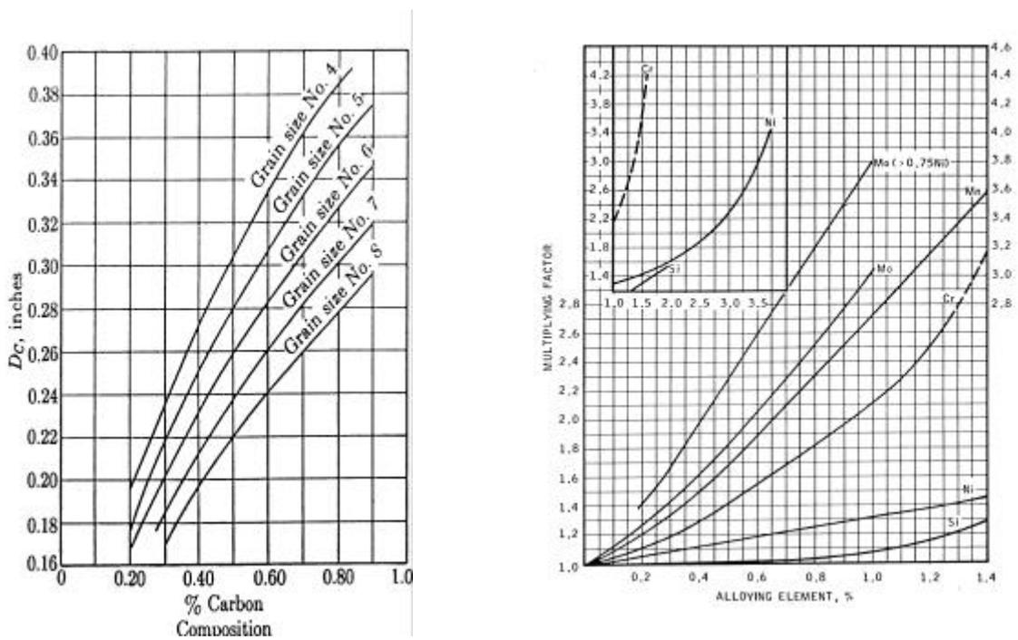
Figure 1. Base diameter,carbon content/grain size      Figure 2. Multiplying factor, element
