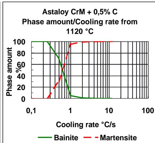
Figure 10 Phase amount, Astaloy CrM + 0.4% C Figure 11 Phase amount, Astaloy CrM + 0.5% C
