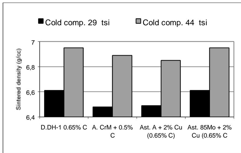
Figure 3. Sintered density, cold compaction.
