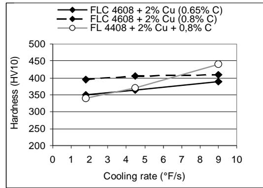
Figure 5. Hardness vs cooling rate
