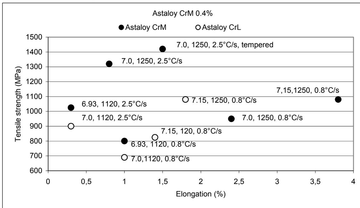
Figure 3. Influence of processing on Astaloy CrM 0.4% C and Astaloy CrL 0.6% C. Denoted in the figure are density, sintering temperature and cooling rate, 7.0 g/cm<sup>3</sup>, 1120°C, 0.8°C/s.
