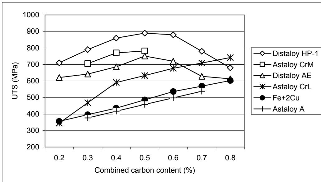
Figure 1. Ultimate tensile strength obtained at different combined carbon contents.
