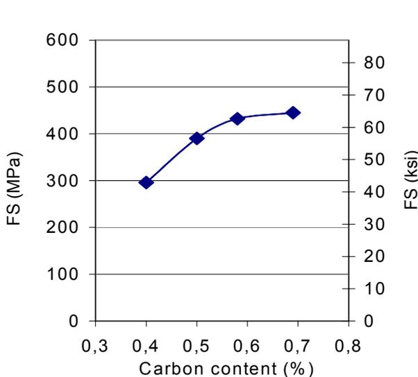
Figure 8. Fatigue strength as a function of carbon content at a cooling of 0.8°C/s.
