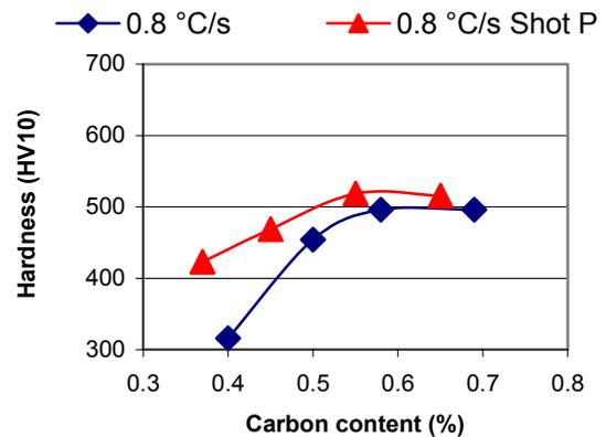
Figure 7. Hardness, HV10, vs carbon content, 0.8°C/s.
