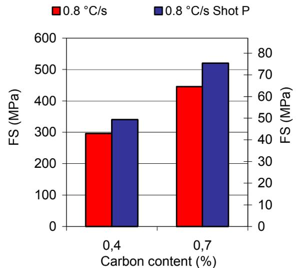
Figure 9. Influence of shot peening on fatigue strength
