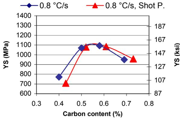
Figure 6. Yield strength vs. carbon content, cooling rate 0.8°C/s.
