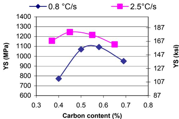
Figure 4. Yield strength vs. carb content, at cooling rate of  $0.8^\circ\text{C/s}$  and  $2.5^\circ\text{C/s}$ .
