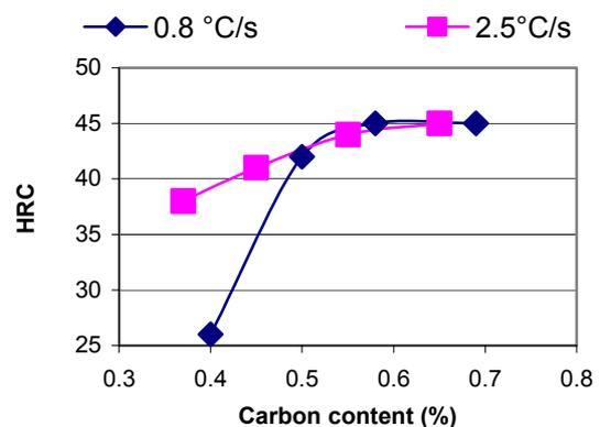
Figure 5. HRC vs. carb content, at cooling rate of  $0.8^\circ\text{C/s}$  and  $2.5^\circ\text{C/s}$ .
