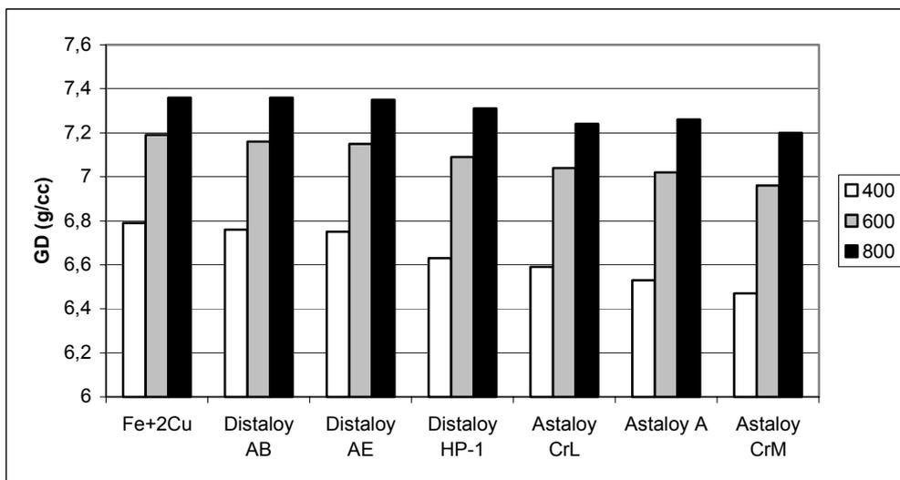
Figure 2. Compressibility for PM grades with 0.6% Kenolube.
