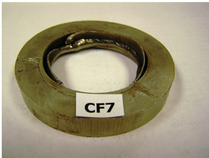
Figure 4: An example of a weld pull test failure showing fracture of the wrought 409L tubing adjacent to the weld. The weld and the PM disc survived the test.
