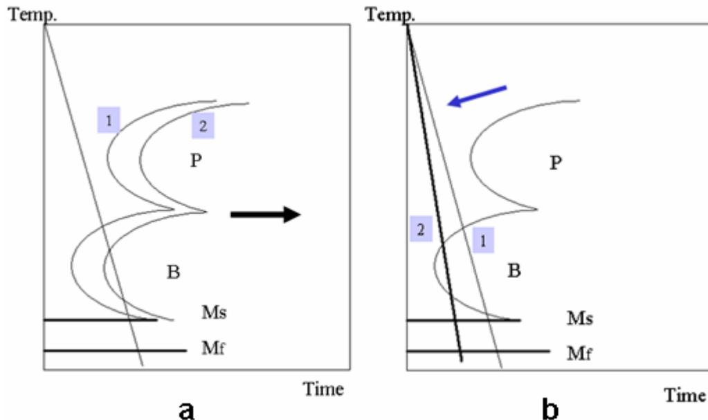
Fig.1 Schematic TTT diagram of PM steel with varying alloying elements (a) and cooling rate (b), where 1 represents low alloying amount in (a) and low cooling rate in (b); and 2 represents high alloying amount in (a) and high cooling rate in (b)
