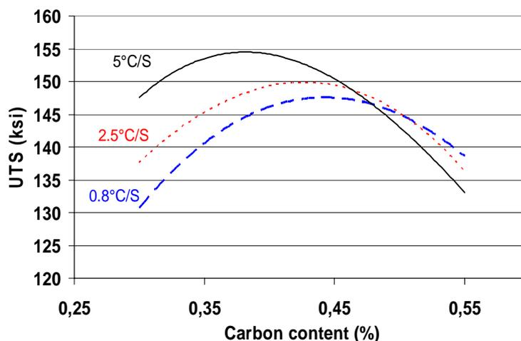
Fig 3 Interaction between carbon content and cooling rate on UTS of Astaloy CrM
