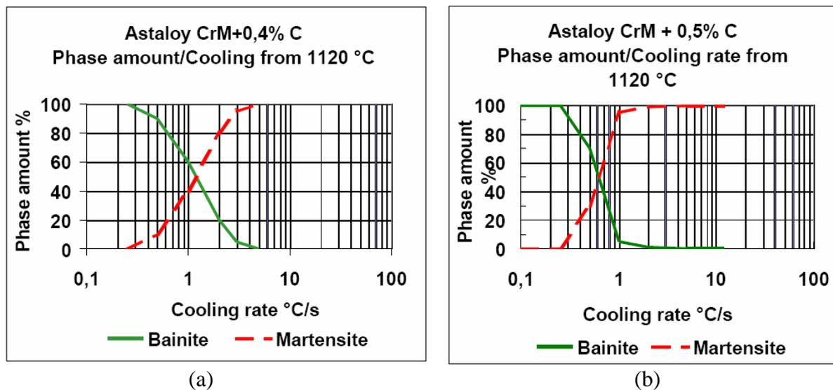
Fig. 2 Phase variation vs. cooling rate for Astaloy CrM + 0.4% C (a) and Astaloy CrM + 0.5% C (b)
