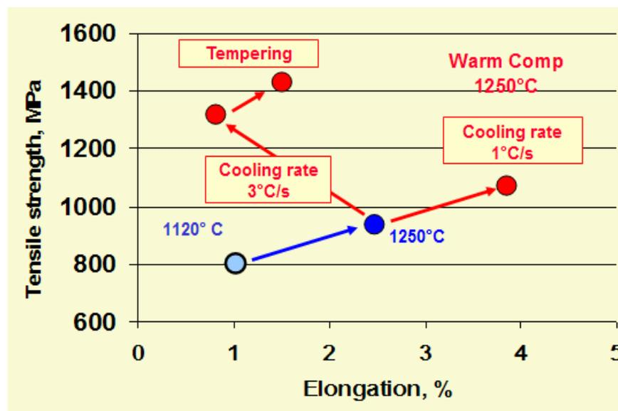
Fig. 4 Properties of Astaloy CrM + 0.4%C under different process conditions
