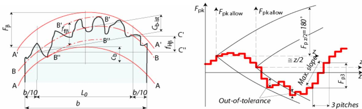
Figure 1 Gear flank line (left) and pitch deviations (right) [11].
