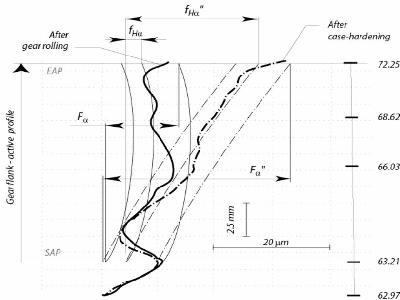
Figure 3. Typical involute profiles of the test gears after gear rolling and after case-hardening. The profile curves belong to the same gear flank, and they were drawn over the scanned profiles from the gear measuring center chart. SAP stands for start-of-active-profile and EAP stands for end-of-active-profile of the gear tooth flank.
