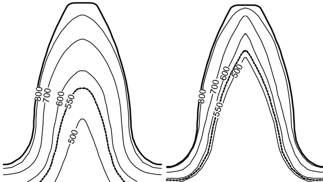
Figure 6. Micro hardness measurement mapping. *Left*: A surface densified P/M gear. *Right*: Reference gear 16MnCr5. The cross section is located in the center of the tooth.
