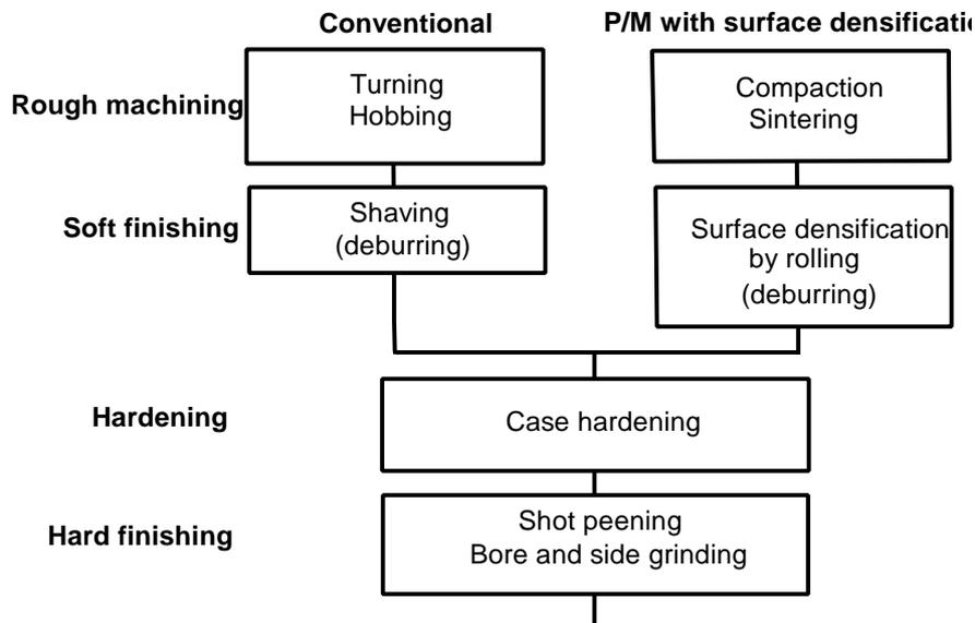
Figure 1. Gear manufacturing sequence for conventional cutting process and for P/M process including surface densification. Washing and transport steps are omitted.
