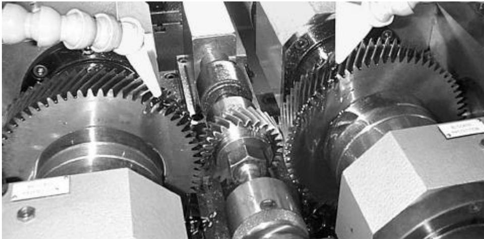
Figure 3. Surface densification of a helical transmission gear using a standard burnishing equipment.
