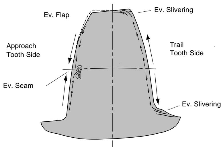
Figure 4. Schematic view of material movement during surface densification [6].
