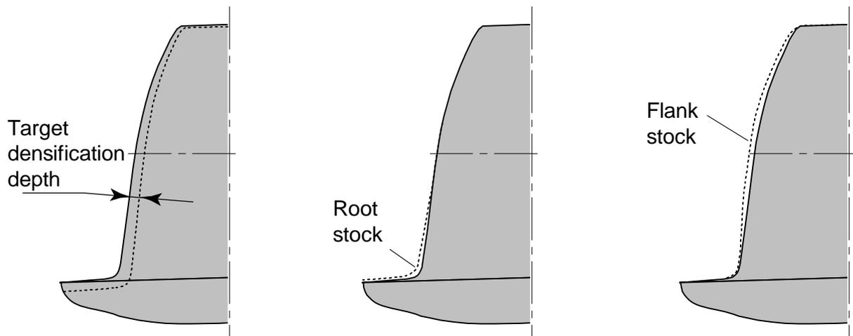
Figure 2. Schematic view of preform. *Left*: Required densification depth. *Center*: Root stock allowance. *Right*: Flank stock allowance.
