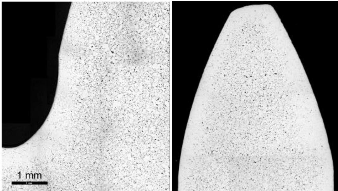
Figure 5. Cross section of a surface densified P/M gear tooth in the as-polished condition. *Left*: Tooth root section. *Right*: Flank and top of tooth. The scale marker is 1 mm.
