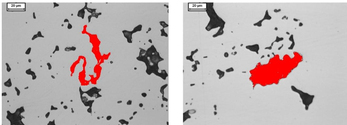
**Figure 9. a. slender pore with large convex area, b. rounder pore with convex area close to actual area.**
