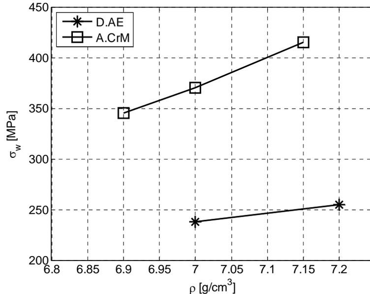
Figure 7. Fatigue strength as a function of density.
