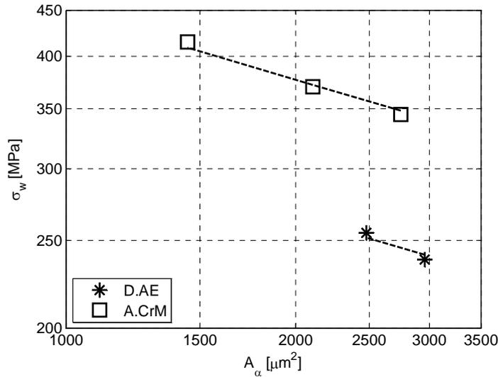
**Figure 8. Fatigue limit as a function of largest pore size.**
