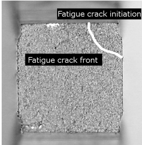
**Figure 3. Crack initiation from the corner.**
