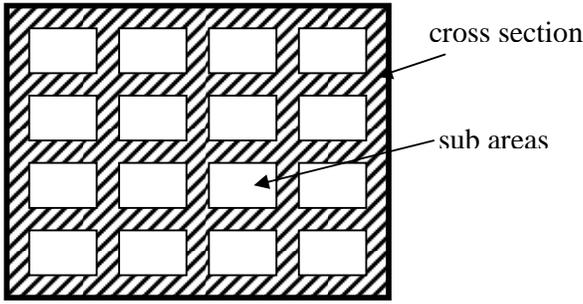
**Figure 1. Cross section of a test bar divided into sub areas.**
