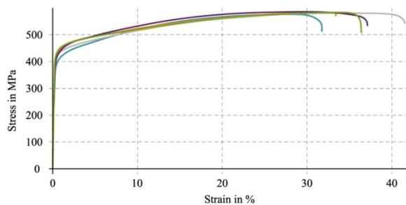
Figure 2a. Tensile strength curves for 316L after laser cladding.
