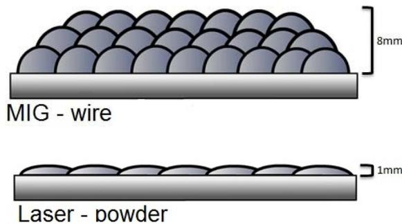
**Figure. 5** Comparison of bead shape
