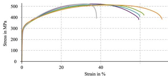
Figure 2b. Tensile strength curves of 316L after GMAW/MIG.
