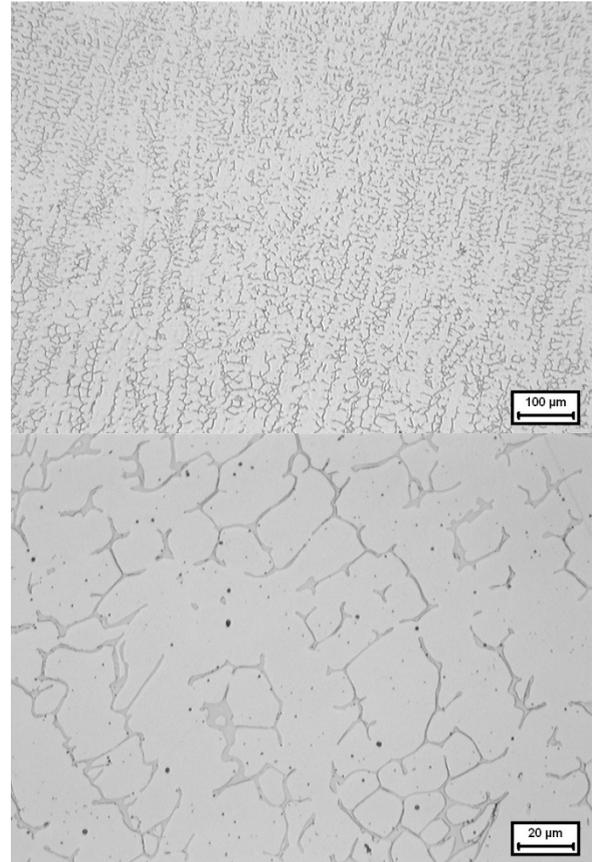
**Figure 4b.** 316L MIG welded etched
