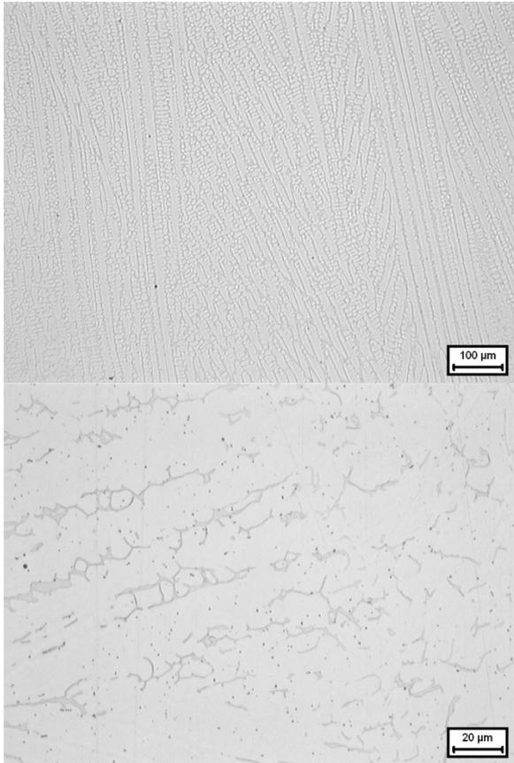
**Figure 4a.** 316L laser welded etched
