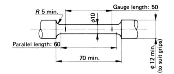
**Figure 1.** Tensile test sample
