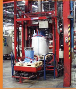
Recently a new installation with a collection funnel for safe emptying of the tube was successfully tested at one of the filling stations in Höganäs, Sweden. The collected powder can now be recirculated as high grade melt stock in Höganäs' own production or externally.
