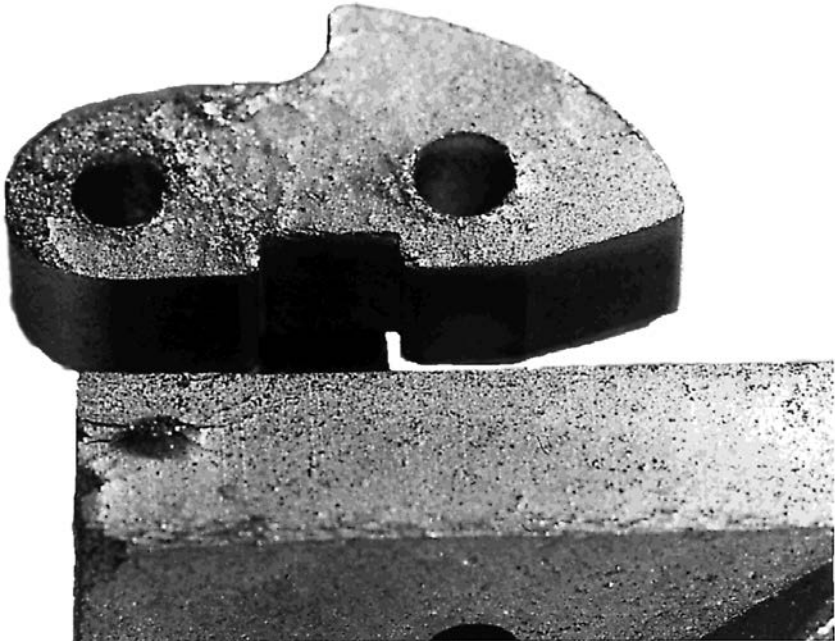
Figure 6.29. Sintered iron powder compact cracked and blistered by carbon precipitation inside pores.
