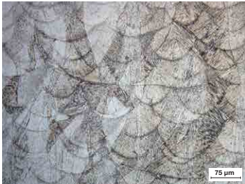
Stress relived - Build direction (40 µm)
