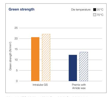
\*Material: ASC100.29 + 1.75 % Cu + 0.8 % C + 0.8 % lubricant. Compaction: 600 MPa.
