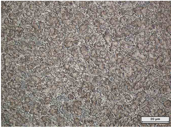
Fine grain martensitic matrix with uniform distribution of hard phase precipitate (etched in Glyceregia).
