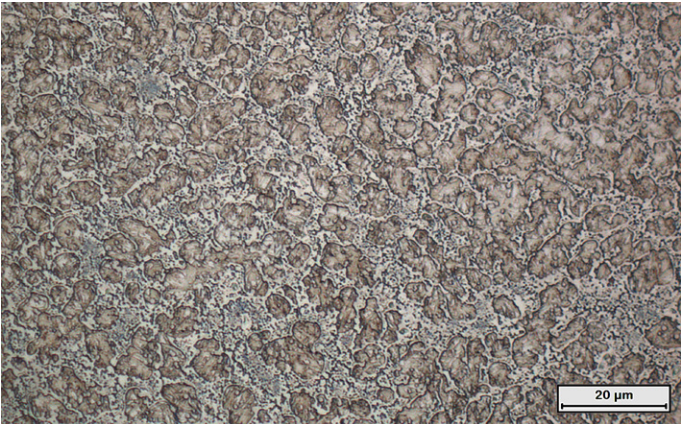
Fine grain martensitic matrix with uniform distribution of hard phase precipitate (etched in Glyceregia)
