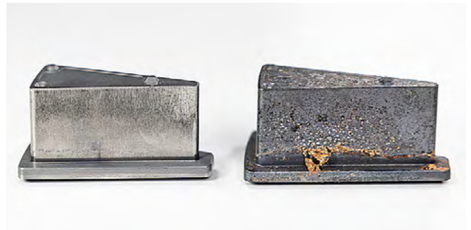
Figure 5. Surface appearance of Somaloy 7P components after heat treatment in controlled O_2 atmosphere (right) and pure N_2 (left).
