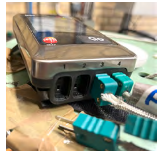
Figure 2. Equipment used to measure the heat-treatment profile inside the component.
