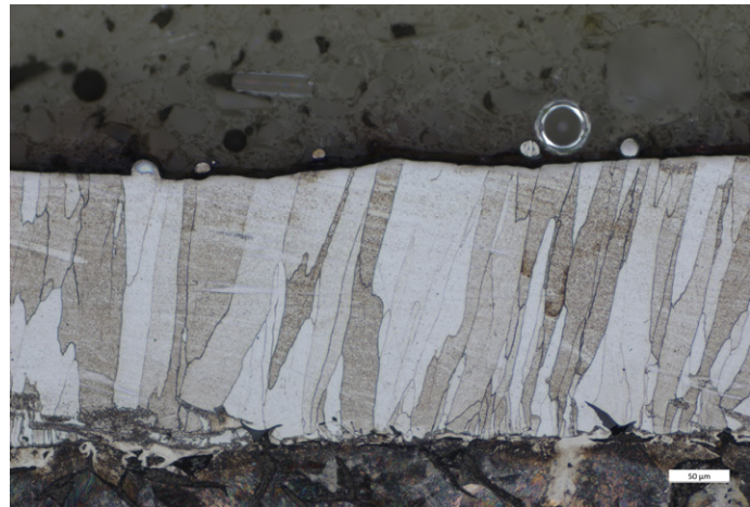
d) 430L as coated at 90 m/min, etched in Vilella. Columnar ferrite grains.
