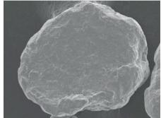
Coarse particle size and a smooth surface facilitates the extrusion of highyield electrodes.
