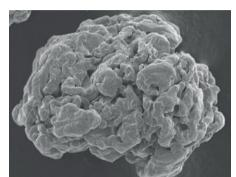
An irregular surface and microporous structure provides a soft and stable arc as well as easy re-striking.
